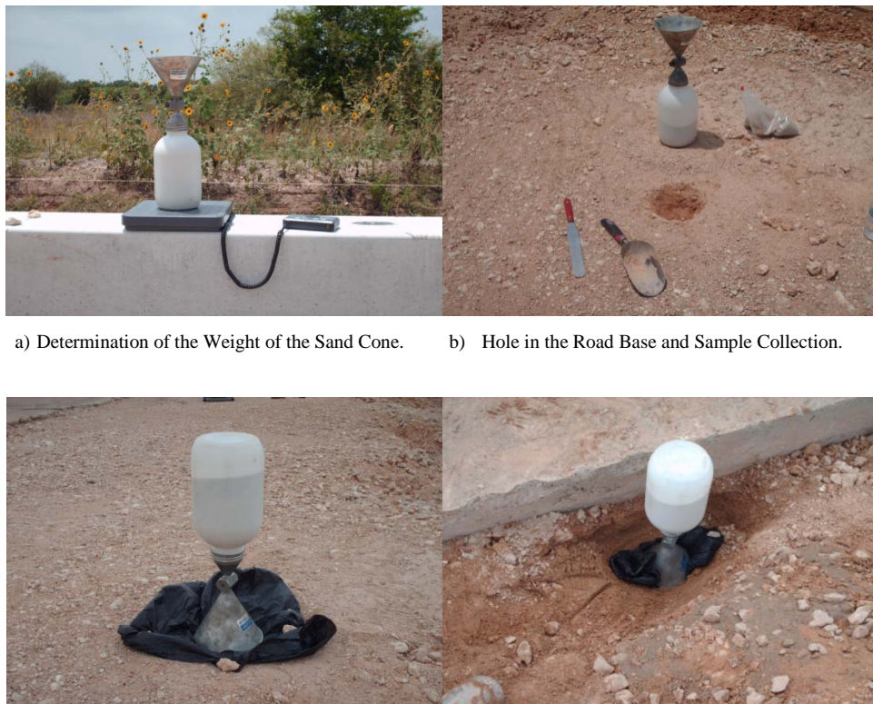
c) Determination of the Unit Weight in the Road Base. d) Determination of Unit Weight in the Clean Sand.
