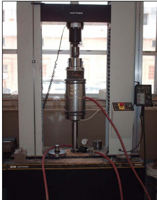
Figure 18. Triaxial Compression Test Conducted on the Clean Sand and the Road Base
