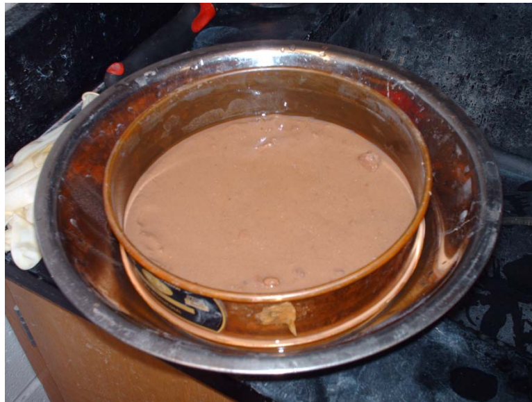
Figure 11. Sand Portion of the Silty Sand Retained in Sieve #200 after Washing
