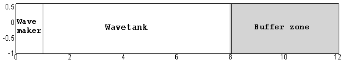
Figure 6 Schematic of buffer zone implementation
