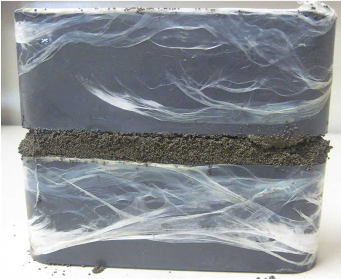
Fig. 3.6—Side and front view of core sample with 8 lb/ft 2 of uncoated proppant
