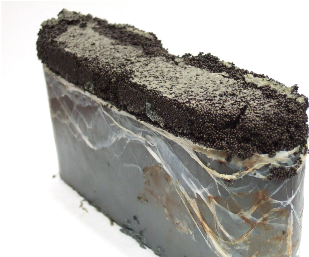
Fig. 3.5—Proppant distribution in the fracture with 8 lb/ft 2 of coated proppant
