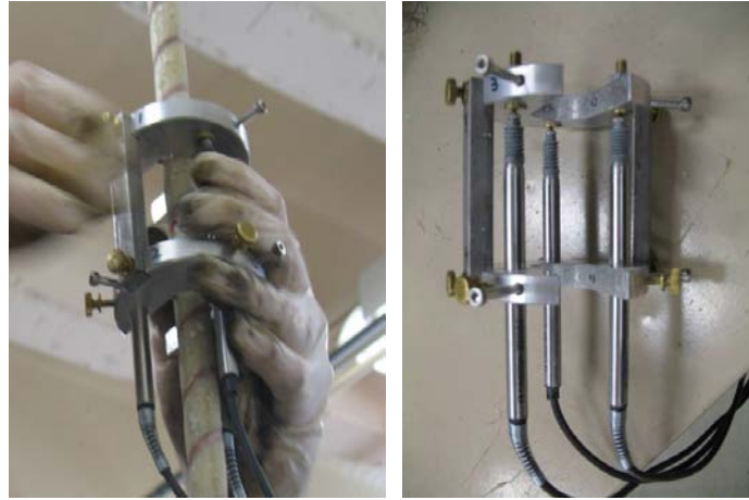
Fig. 9. LVDTs being mounted to GFRP bar (left) and LVDT for MOE (right)
