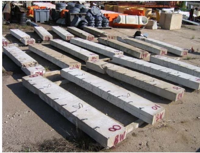
Fig. 4. Concrete beams containing the GFRP reinforcement at the Riverside Campus in Texas A&M University
