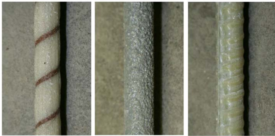
Fig. 5. Surface of each GFRP (V1, V2, and P respectively)
