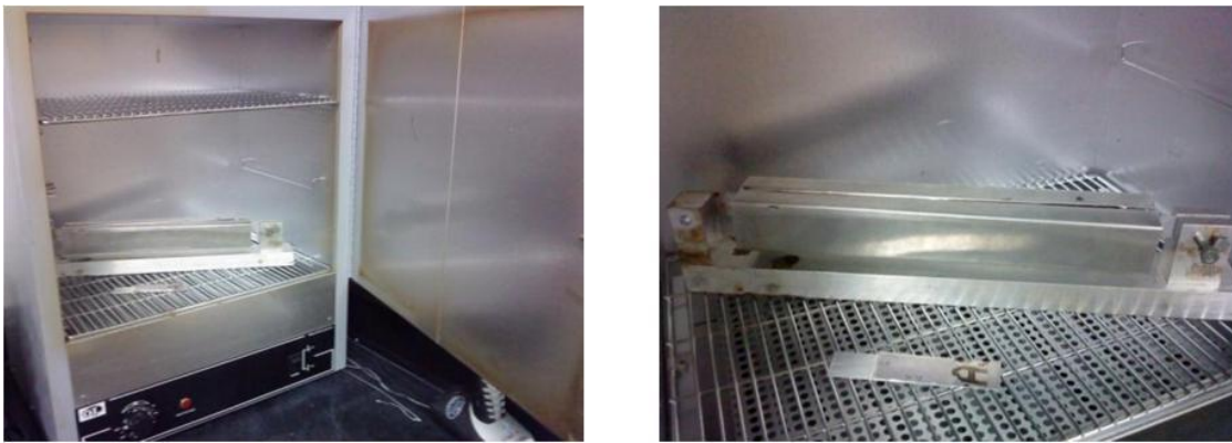
Figure 24. In this test, the twisted spar and the lap shear test panel were simultaneously heated in an oven to find a temperature that softened the locking material without annealing the spar. The locking polymer had to form a good bond with the aluminum plates.
