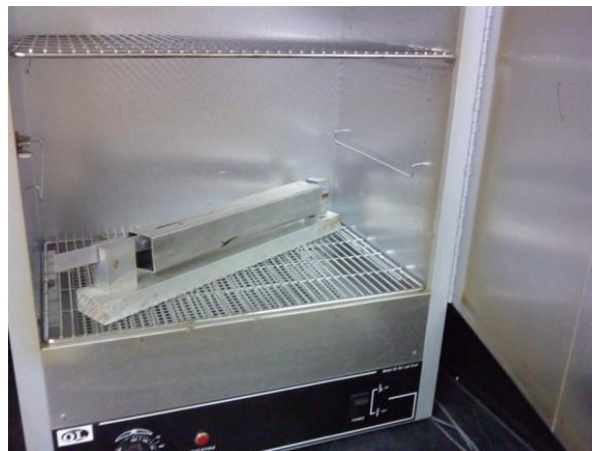
Figure 35. Apply heat 288°C (550°F) to the twisted spar with placing on the locking material during 15min.
