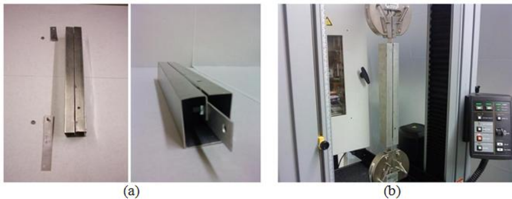
Figure 21. (a) Tabs connect to the spar section's flanges with bolts and nuts. (b) Tensile test machine fixed with the tabs show relation between force applied and displacement.
