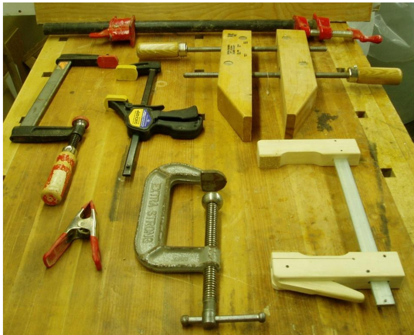
Figure 11. Top row: Pipe clamp / 2nd row from top: F-clamp or bar clamp, one-handed bar clamp, wooden hand screw / 3rd row: spring clamp, C-clamp, cam clamp [19].
