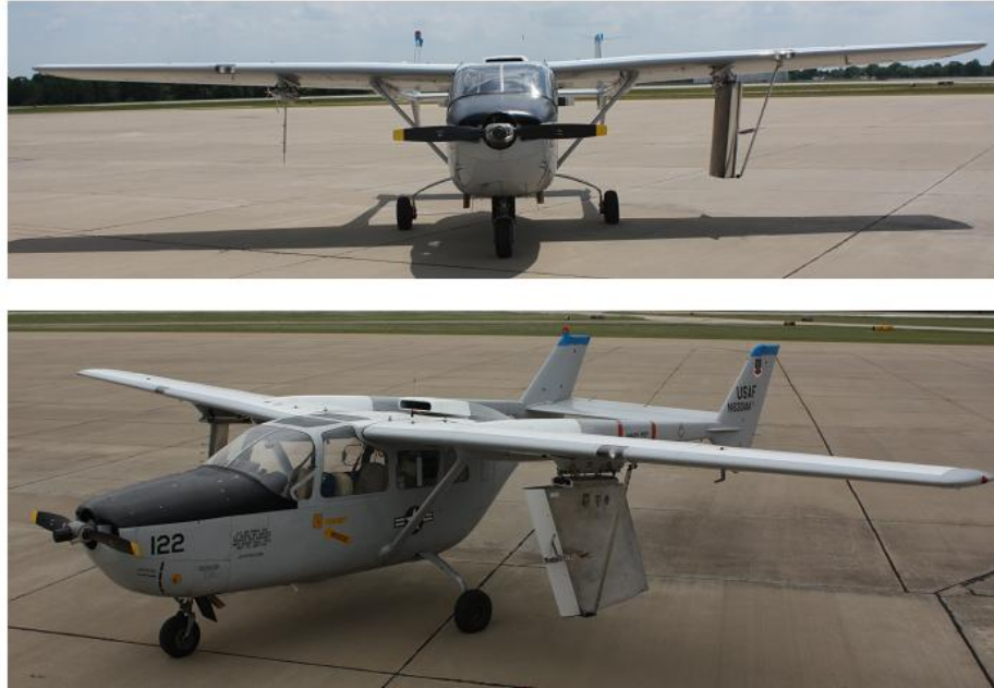
Fig. 3 O-2A with SWIFT model vertically mounted on port wing.
