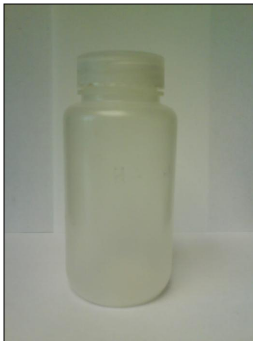
Figure 3.2 Reactor (250-mL polypropylene bottles) used to determine kinetic parameters in the pH-activated experiments.
