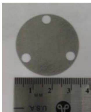
Fig. 2. Photograph of titanium disk measuring 3.4 cm in diameter.
