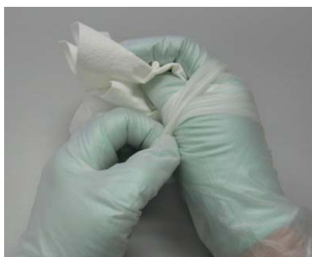
Fig. 8. Removing the outer vinyl gloves while keeping the wipe inside.
