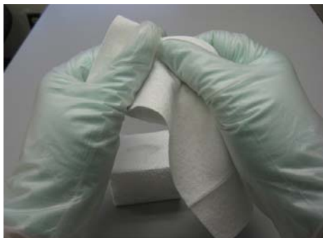
Fig. 21. Simulation of smearing the disk source for removable ^{73}\text{As}/^{74}\text{As} material.
