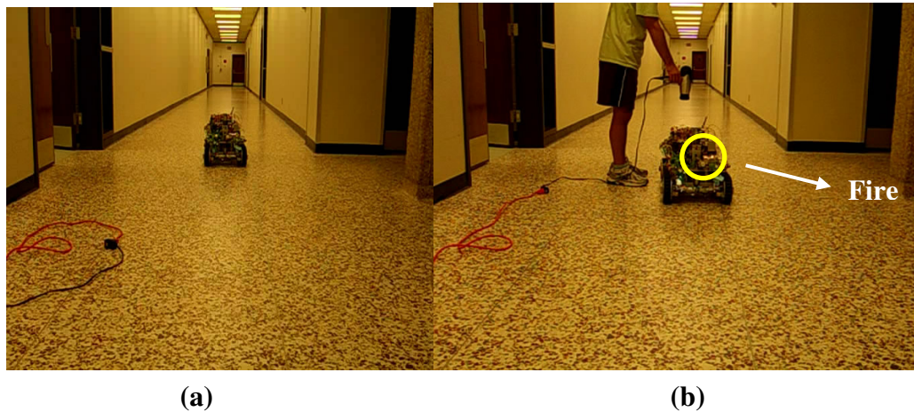
Figure 54. Mother Vehicle find fire and stop test. (a) MV stays in the hallway. (b) MV finds and approaches.
