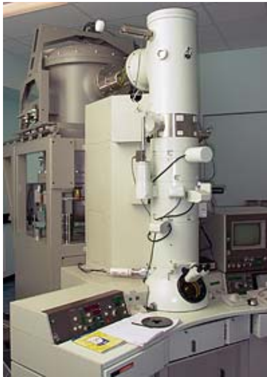
Fig. 30 JEOL 3000F, transmission electron microscope.
