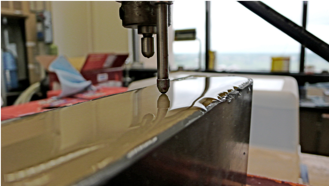
Figure 4.3 Thickness Verification by Micrometer
