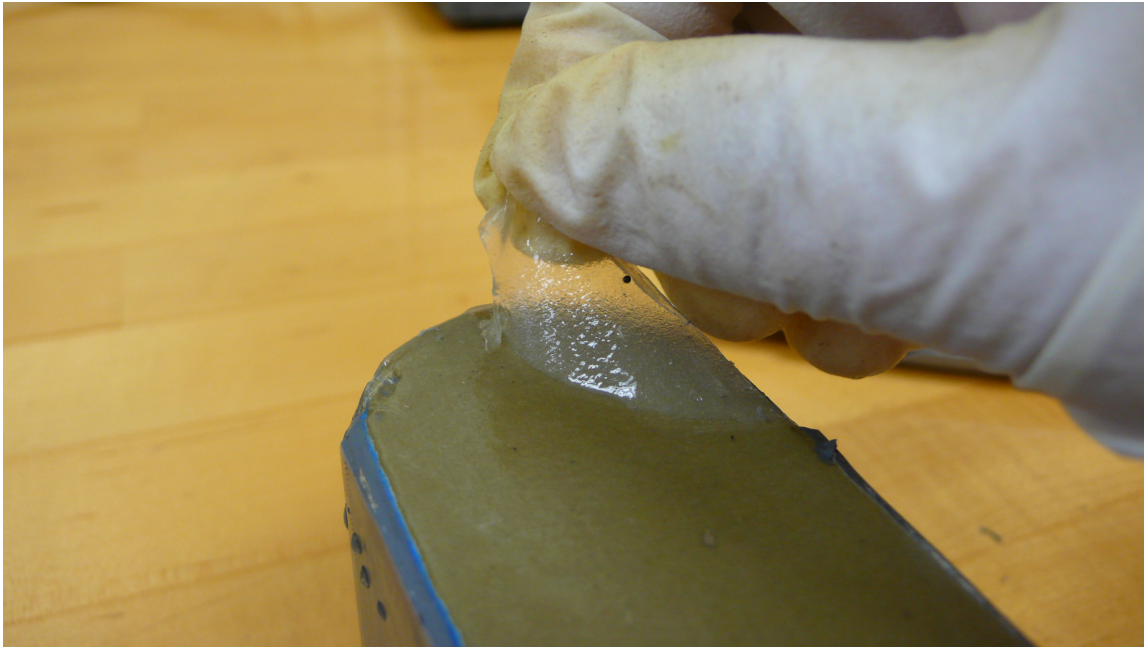
Figure 4.8 Stretched Filter Cake after 200 \text{ s}^{-1} Shear Rate Erosion
