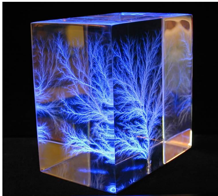
Fig. 3.16— Electron paths of irradiated sample (source: Stoneridge Engineering).
