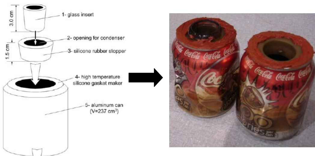
Fig. 2.17 —Previous reactor design (Daniyar Zhusspov 2006).
