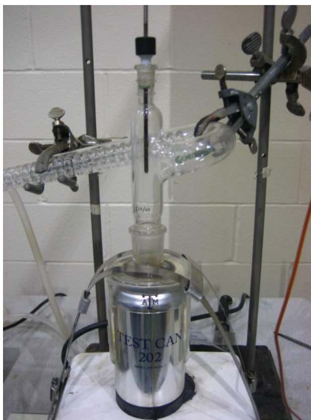
Fig. 2.20—Custom made apparatus provides uniform pressure to seal the gasket in the contact area. However, aluminum can start collapsing when the fluid reaches high temperature because of thermal stress.
