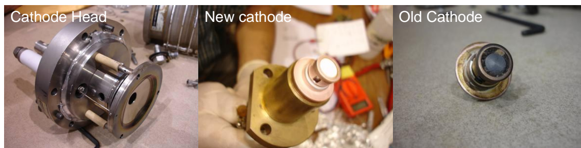
Fig. 2.4—Cathode head, new cathode, and old cathode.
