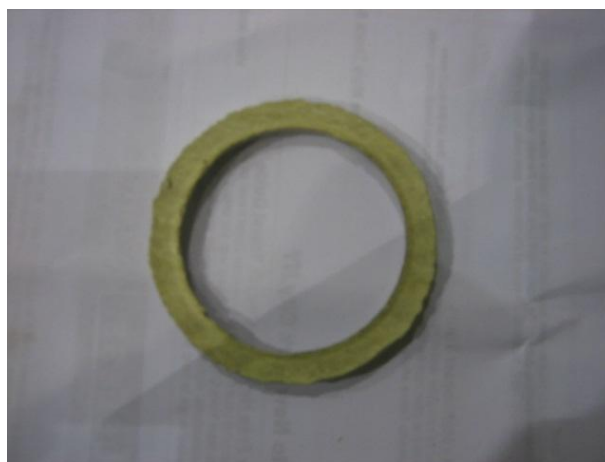
Fig. 2.19 —Custom made gasket “style -760” can stay with maximum temperature of 700 °C.
