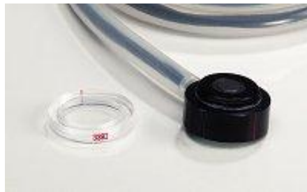
Fig. 2.7—The Markus chamber has volume of 0.055cc and measure maximum dose of 50Gy. The membrane material is polyethylene of 0.03 mm thickness. The guard ring borders the measuring volume.
