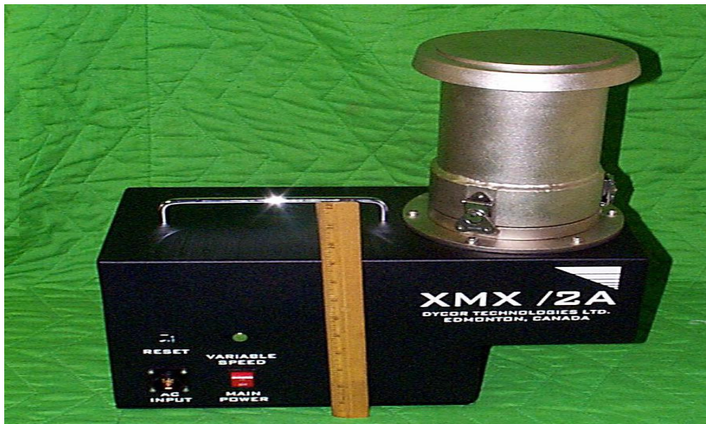
Figure B.5a Three-stage aerosol concentrator XMX/2A (Kesavan et al., 2008)
