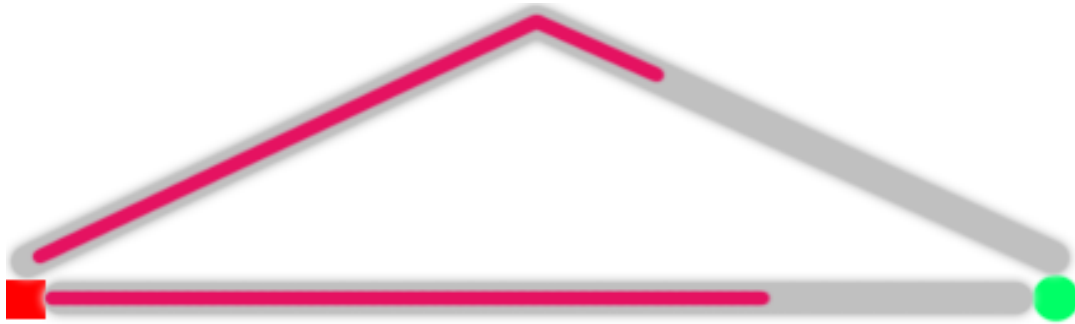
Figure 3: Two pheromone paths are shown, one longer than the other. The two pink lines are the same length, visually demonstrating that shorter pheromone paths allow for faster transit between nest and food than longer paths. This will cause shorter paths to strengthen and longer paths to fade away over time.
