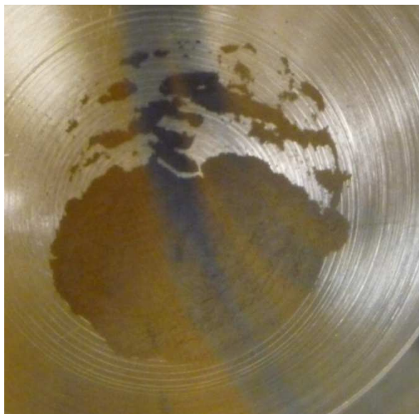
Figure 4-10 Powder after being milled in the Wig-L-Bug (sintered chunks/no hydride DU was removed)
