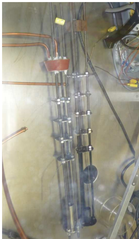
Fig. 3-10 The alpha phase sintering experiment reaction vessel (right) lying next to the hydride reaction vessel (left) on the glovebox floor.
