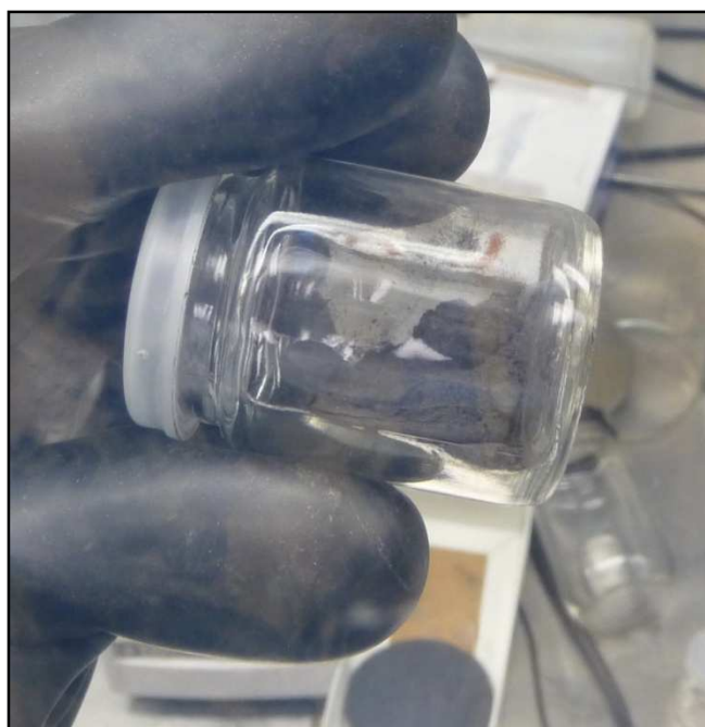
Figure 4-8 Break down of sintered powder after shaking the container
