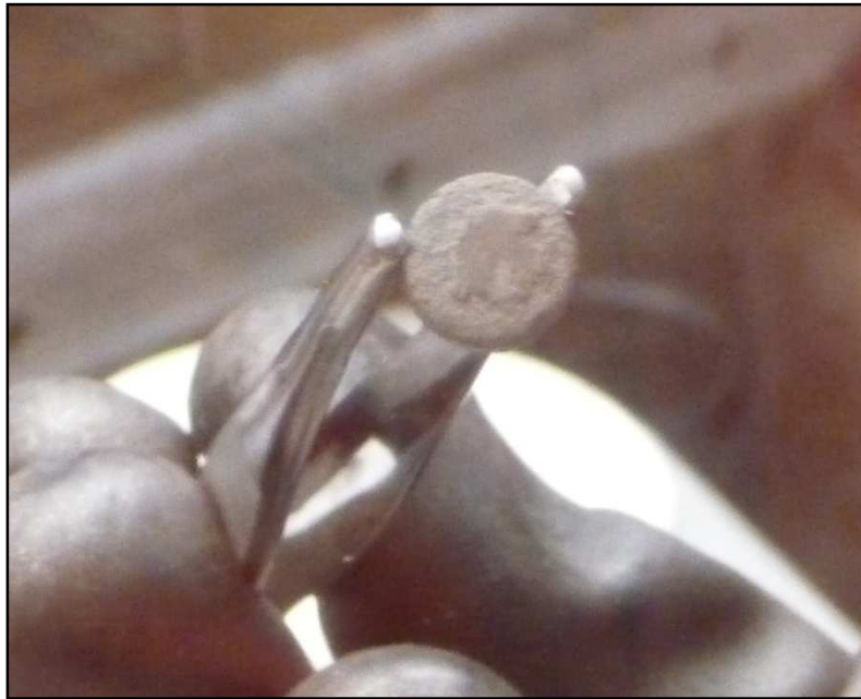
Fig. 4-35 Pellet 9 (DU-10Zr Wt %) post experiment
