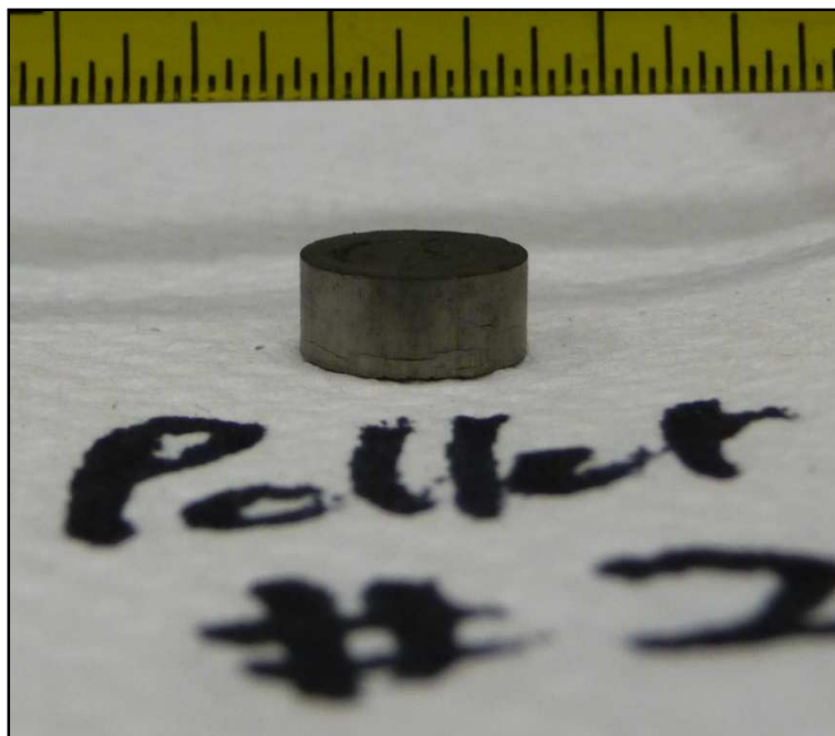
Fig. 4-22 Pellet 2 post sinter
