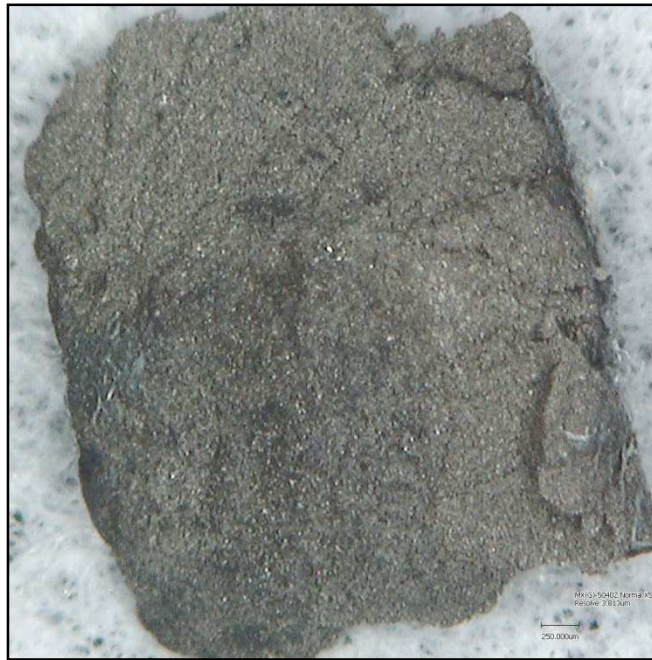
Fig. 4-16 DU powder sintered during dehydrating at 50X
