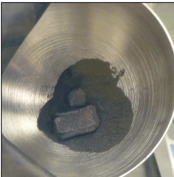
Figure 4-9 Powder, sintered chunks, and non-hydrated DU ground with mortar and pestle
