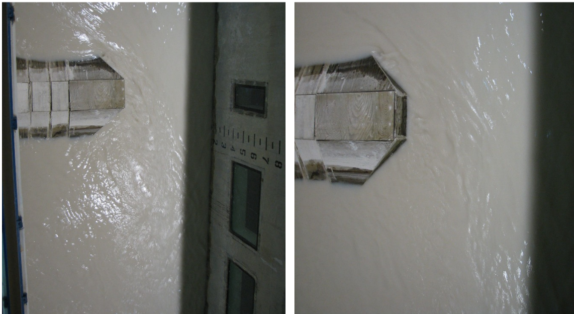
Figure C.25. Flow pattern around abutment of case 12B (flow from top to bottom)
