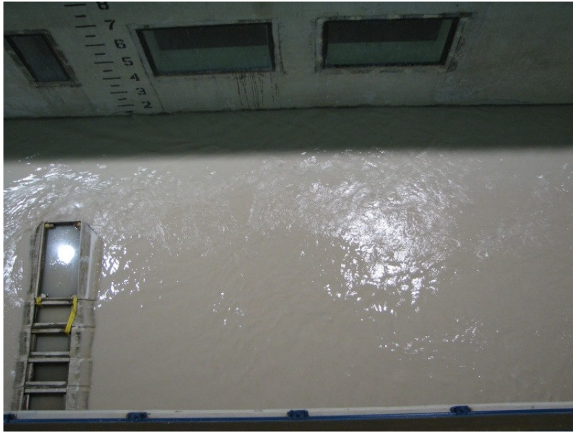
Figure C.31. Flow pattern around abutment of case 15 (flow from left to right)
