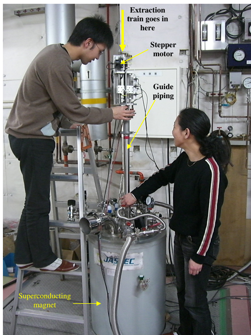
Figure II.18. 18 Tesla extraction type magnetometer in High Field Laboratory for Superconducting Materials, Institute for Materials Research, Tohoku University, Japan.
