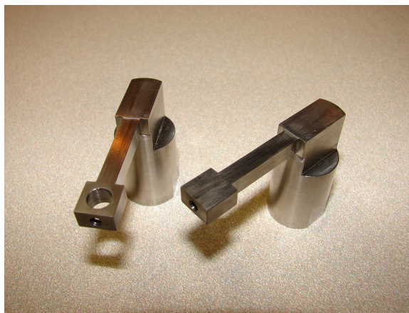
Figure II.2a. Actual photograph of the custom narrow grip heads for compression.
