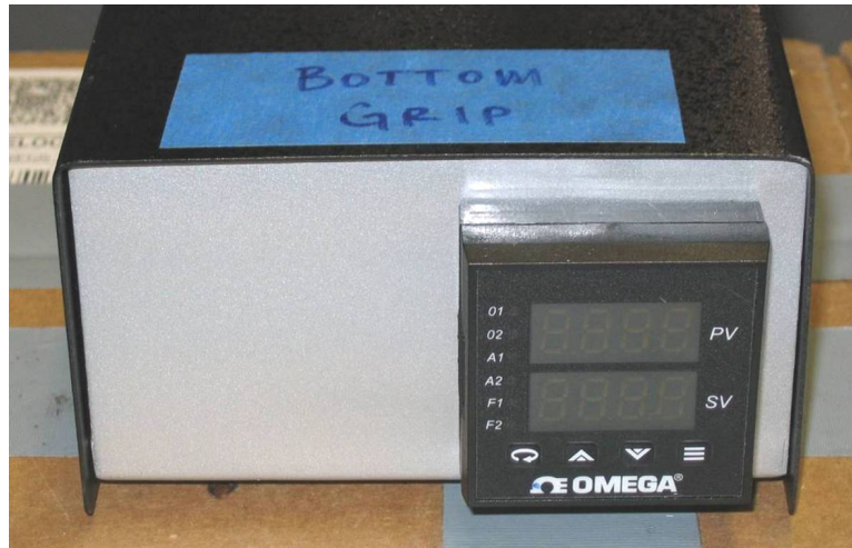
Figure II.8. Temperature controller used to control thermal management system.
