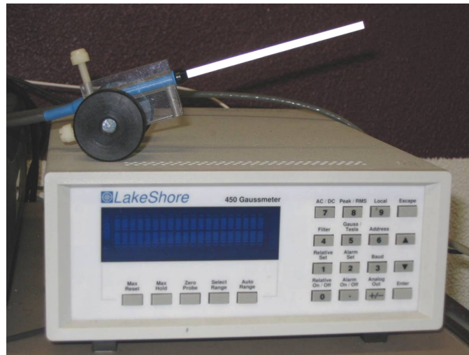
Figure II.10. LakeShore 450 Gaussmeter and cryogenic transverse Hall Probe used to provide feedback and control the electromagnet.
