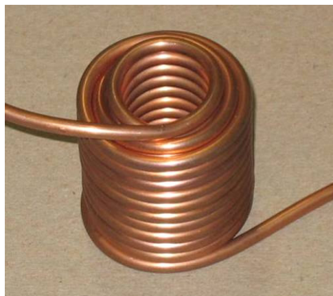
Figure II.5. Cu coil windings used to channel liquid nitrogen.
