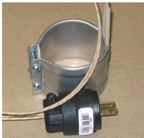
Figure II.6. Watlow thin-band mica heater used to heat compression grips.
