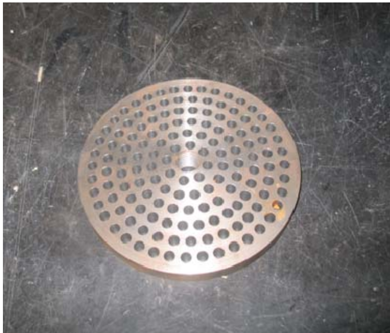
Figure A-4 cast iron conical grate with 144 of 0.25 in drilled holes
