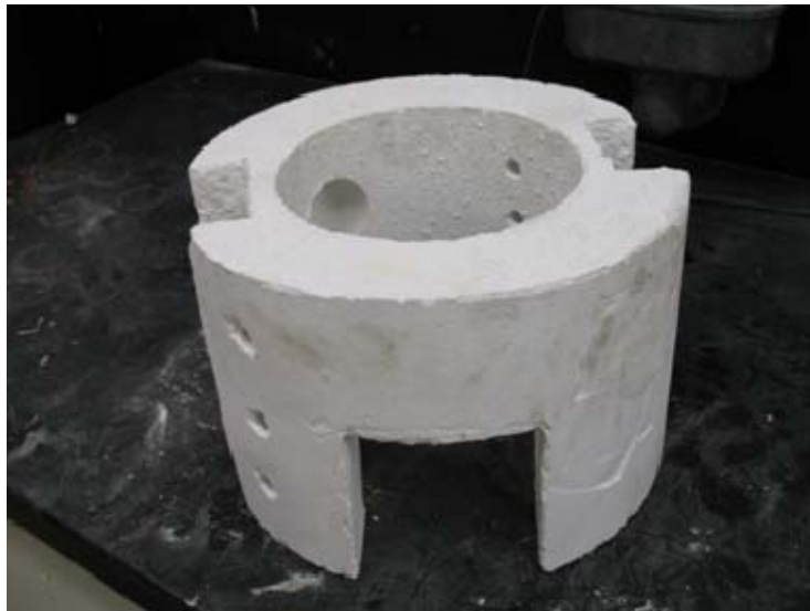
Figure A-1. Combustion chamber built in castable alumina with inner and outer diameter of 6 in and 10 in respectively
