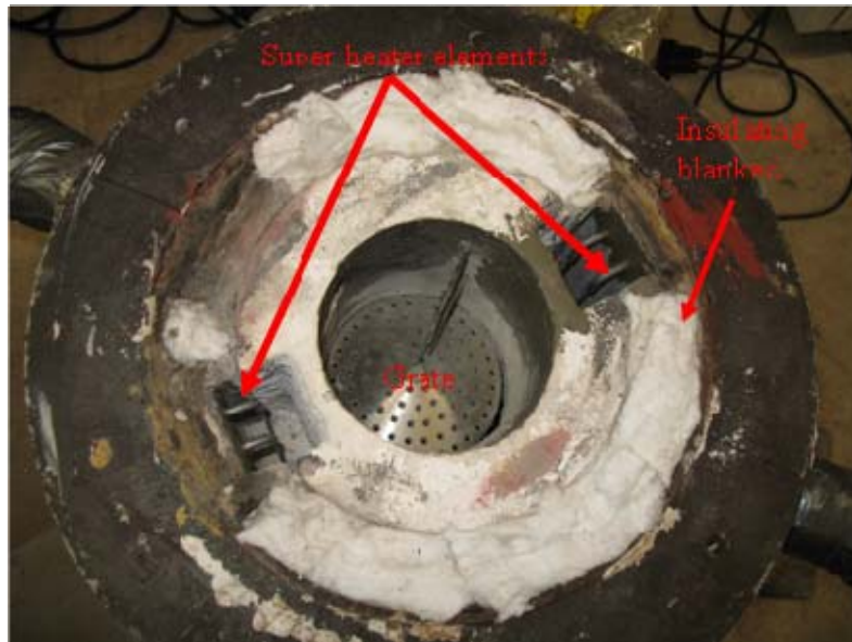
Figure A-3. Combustion chamber with two super heater elements and cast iron conical grate
