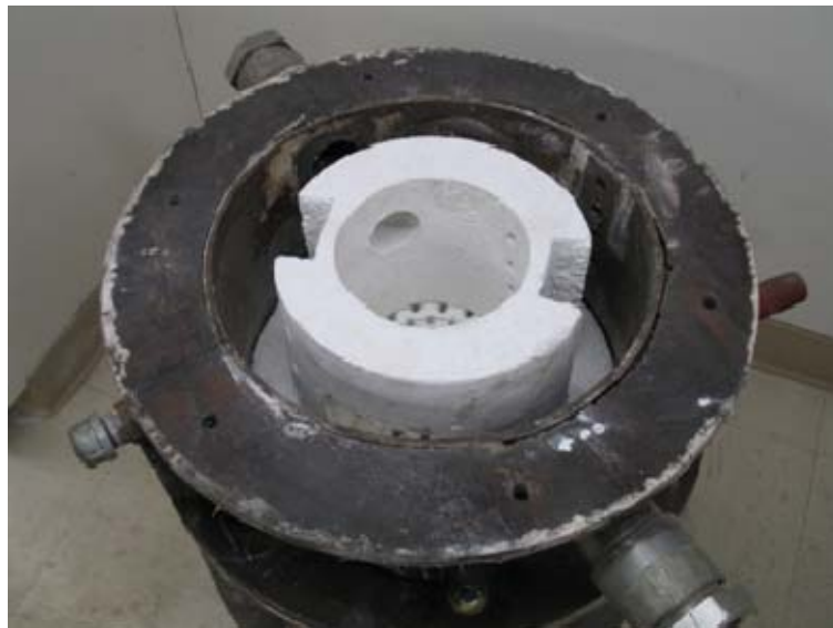
Figure A-2. Combustion chamber and outer steel tube with a inner diameter of 13.5 in
