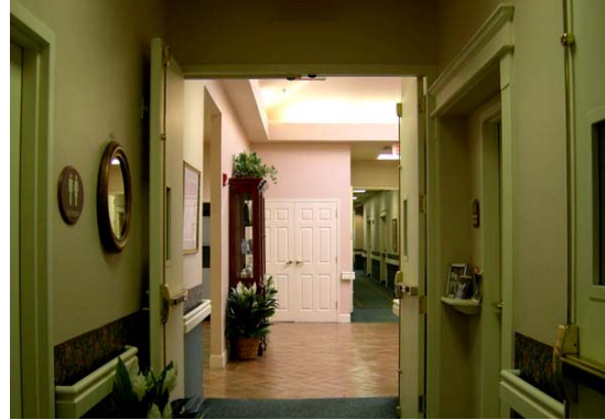
Figure A-3 Changing the axis of the corridor to break the long sight line of the path
