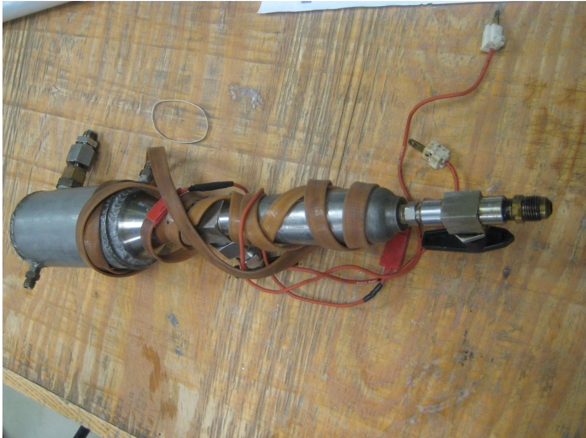
Fig. 3.6—Two-stage separator with electric heater tape wrapped around it.
