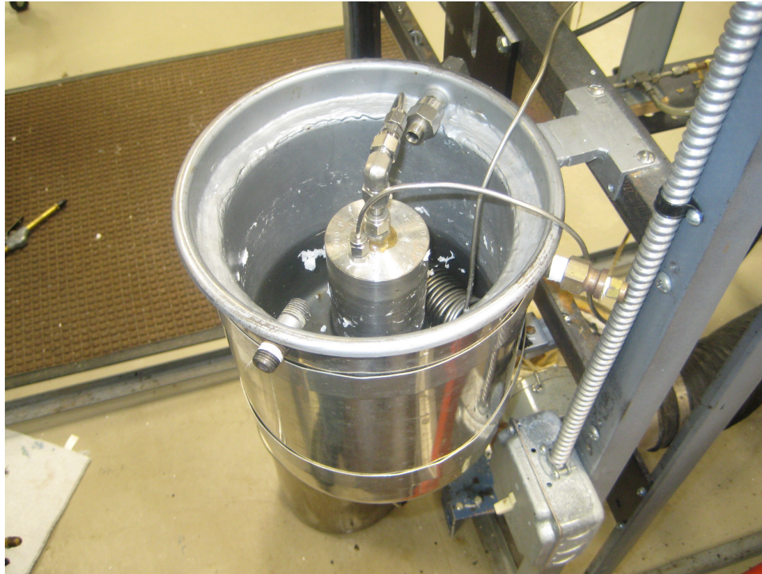
Fig. 3.7—Condenser unit to cool and condense liquids from produced gases.
