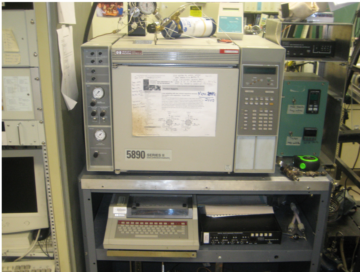
Fig. 3.9—HP 5890 Series II gas chromatograph, HP 3966A integrator and VICI sequence programmer.
