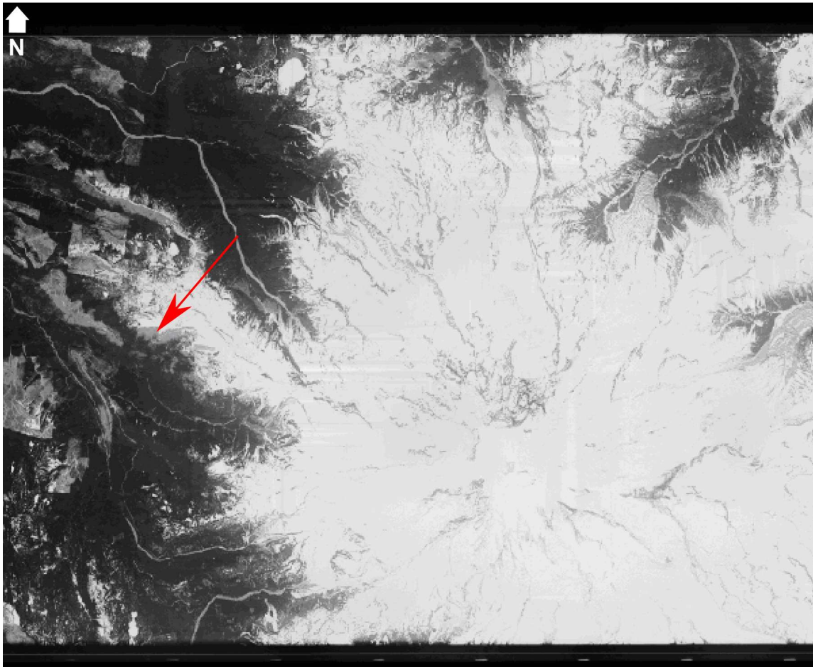
Figure 3-4: Partial strip (panchromatic) of scanned film from the KH-4B CORONA satellite that was used to map trees (~18 km x 13 km displayed above). The tip of the red arrow identifies the ridge burned by the 1930 fire (Source: USGS).
