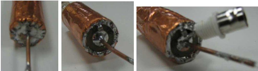
Figure 50: Showing the two ends of a fabricated balun. (a) Bottom end of balun (b) Top end of balun (c) BNC connector across capacitor.
