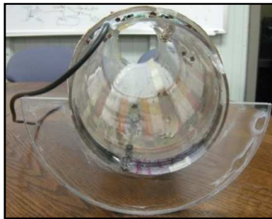
Figure 19: Centering mechanism attached to the birdcage coil.
