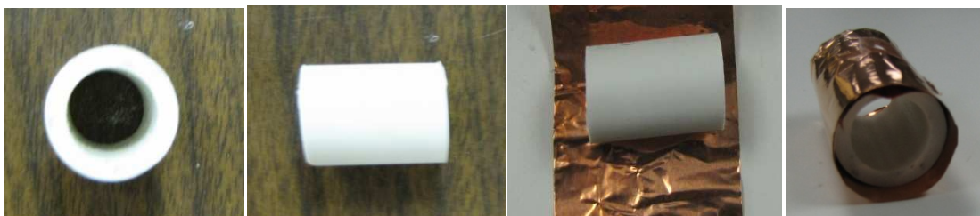
Figure 49: Stepwise construction of a balun. (a) Hollow tube top view (b) Hollow tube side view (c) Hollow tube placed in copper sheet (d) Copper sheet wrapped around the hollow tube.
