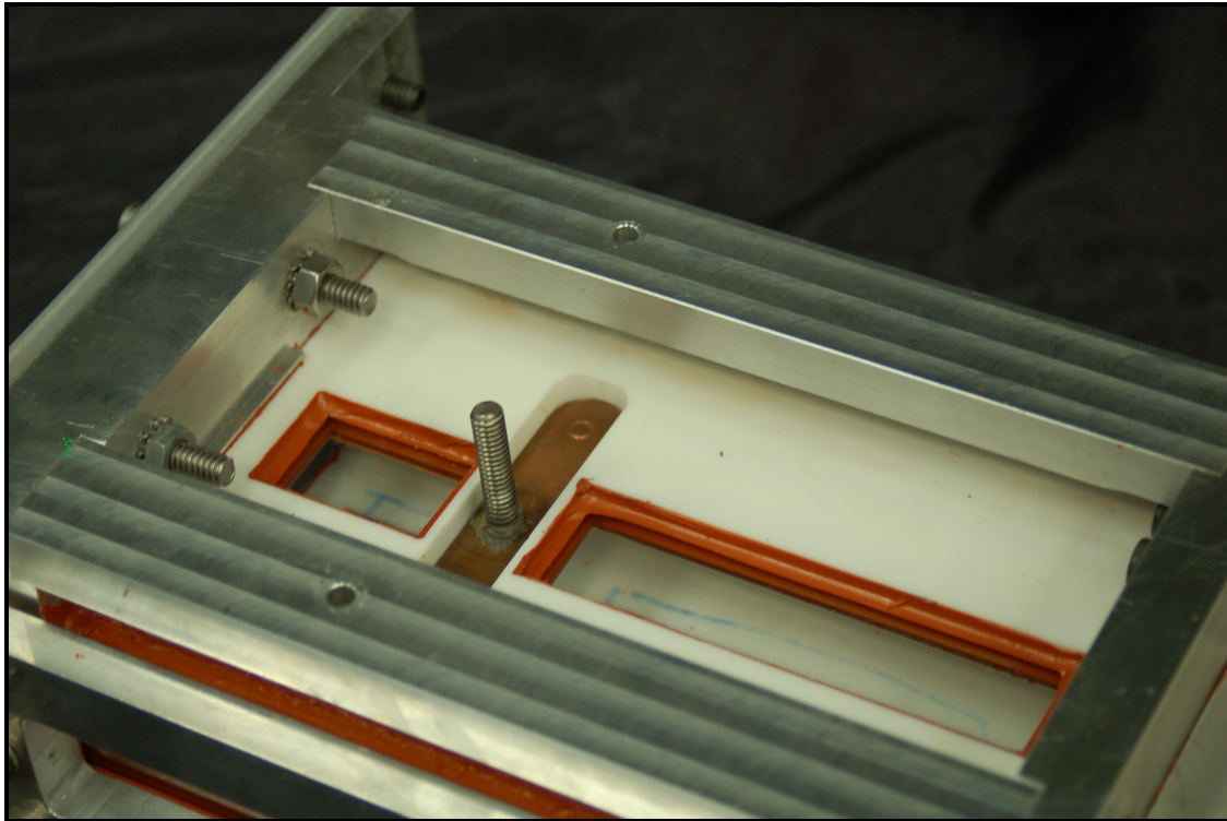
Fig. 2.14 Closeup of Macor plasma discharge section of subsonic test section (digital photo)
