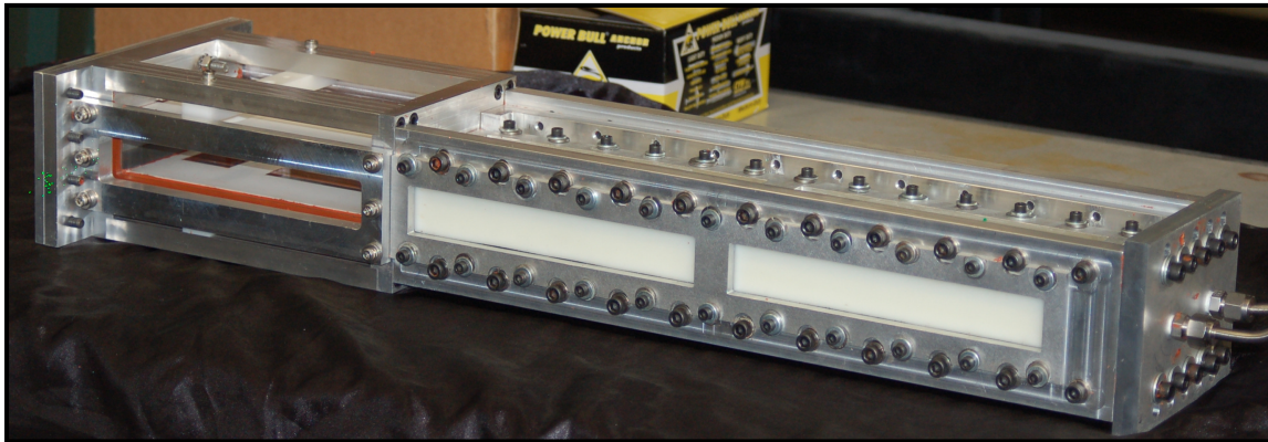
Fig. 2.12 Subsonic test section leak testing assembly (digital photo)
