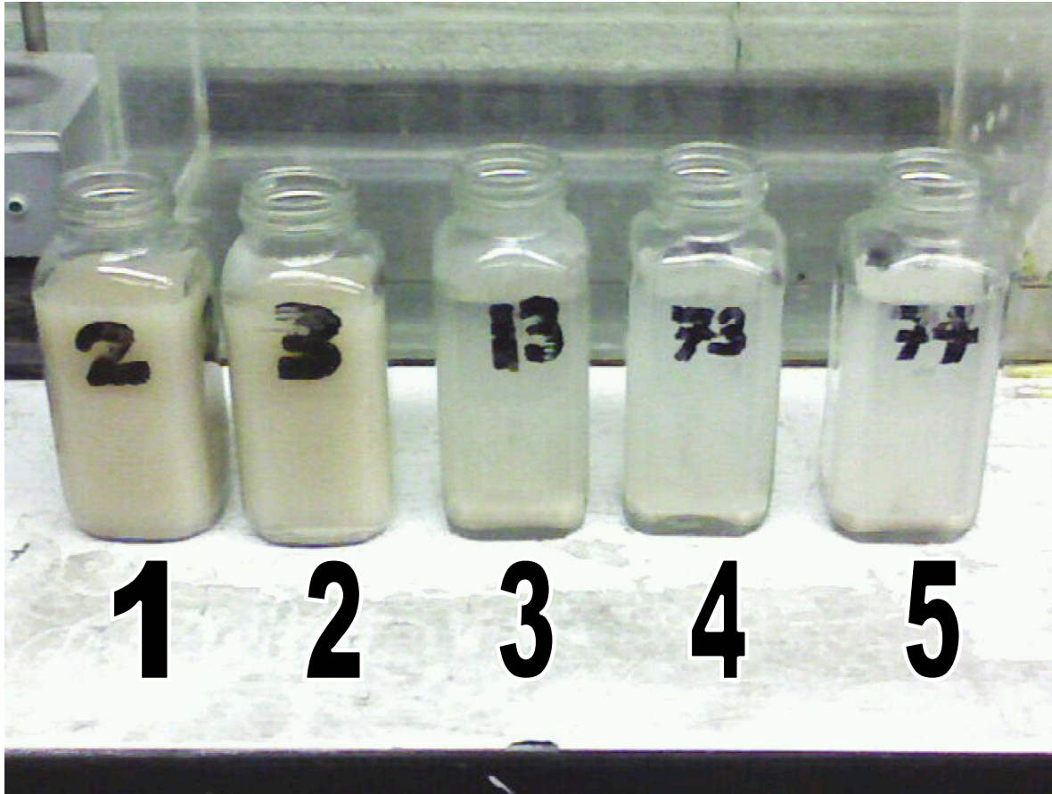
Fig. 2.3. Photograph of sample “suspensions” at the time to withdraw the <2 \mu fraction pipetting. Sample treatment followed Procedure Three. Composition of prepared samples 1 through 5 are given in Table 2.1.
