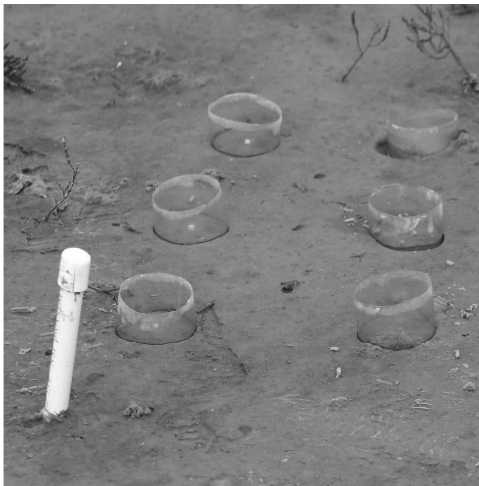
Figure 16: Photograph showing the experimental set-up at one of the three stations used in the nutrient enrichment study. The three cores on the left were amended with slow release fertilizer sticks and the three cores located to the right were the control samples.
