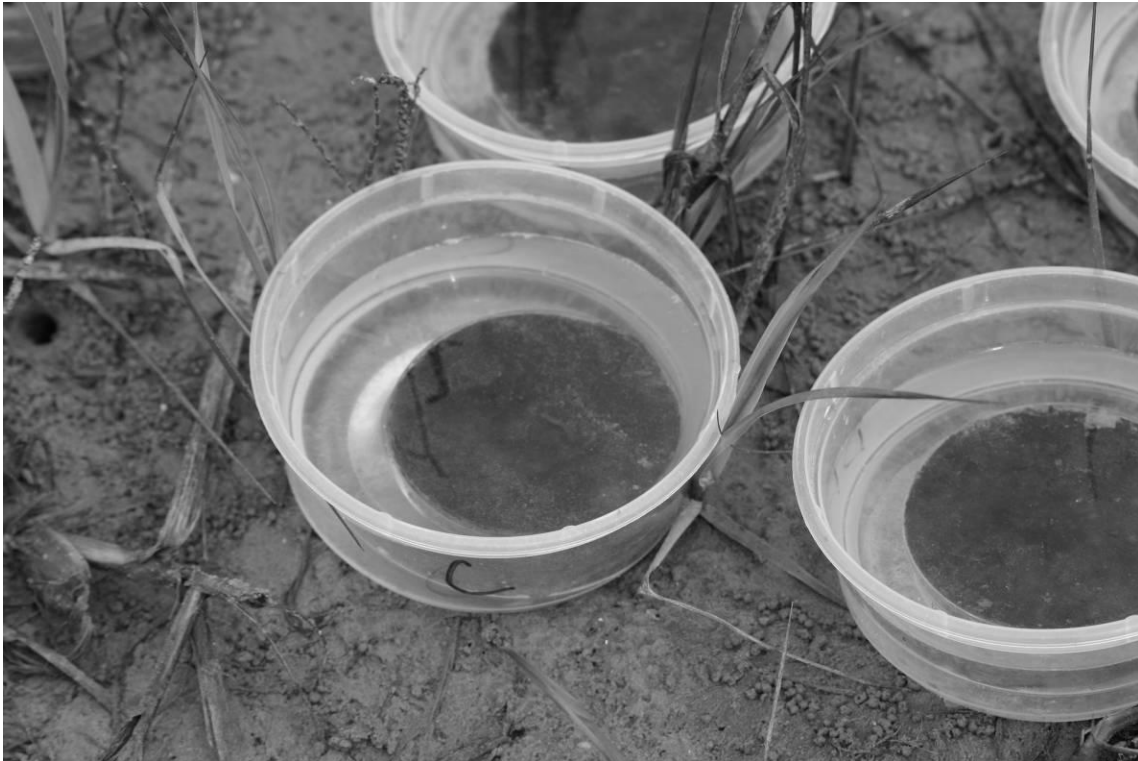
Figure 12: Container setup for the salinity bioassays. The petri dish was used to collect the sediment and then placed in a shallow container filled with seawater in the correct salinity (control = ambient seawater, DI = deionized water, DL = ambient seawater diluted in half with deionized water, 25% = 25% increase above ambient seawater, and 50% = 50% increase above ambient seawater). The water in each container was exchanged daily with newly-mixed treatment water.
