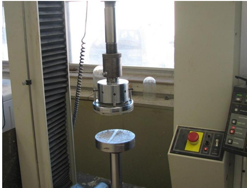
a) Compression Machine Used to Perform Single Aggregate Testing (Model: INSTRON 5583)
