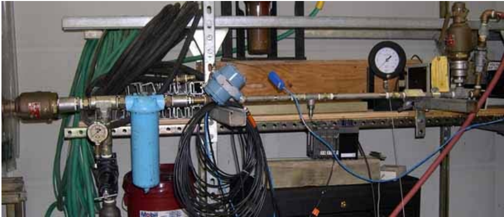
Figure A4. Air control system
