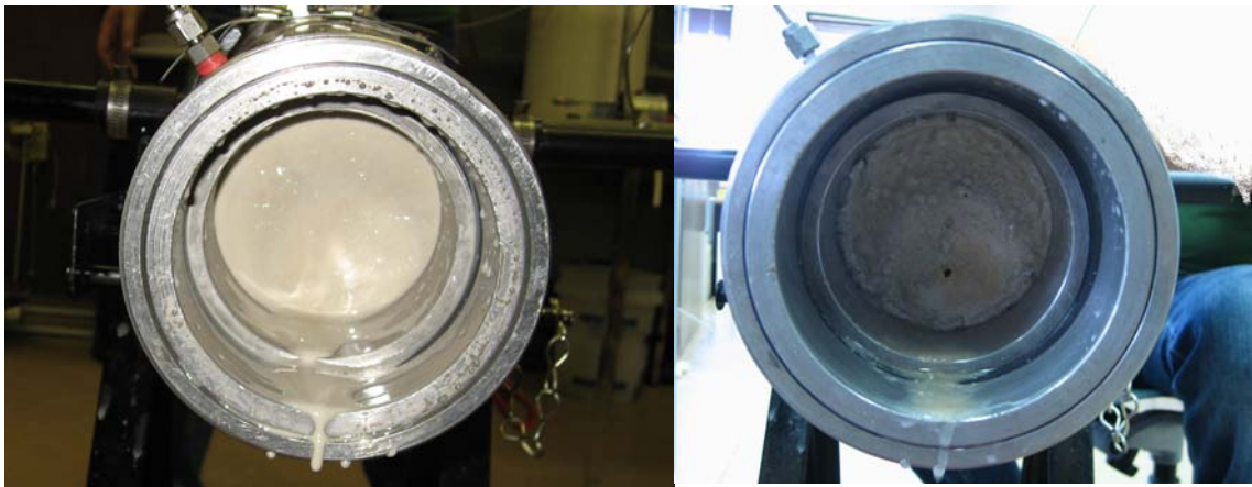
Figure 5.1 Core sample C1 (a) after filter cake deposition, and (b) after the acid jetting treatment
