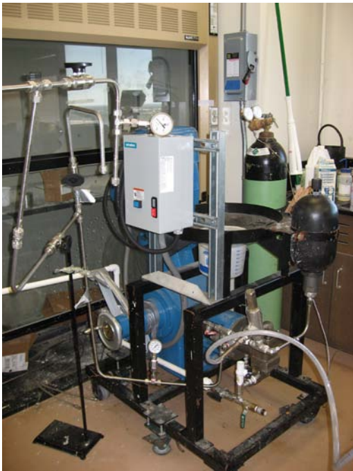
Figure 3.9 Picture of drill-in fluid pump
