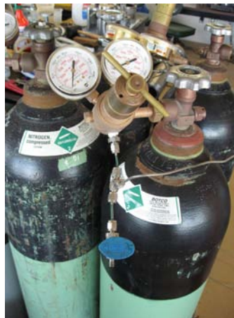
Figure 3.21 Nitrogen tank with pressure regulator
