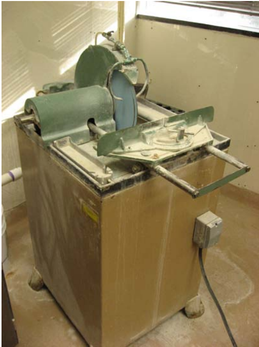
Figure 3.1 Abrasive cut off machine
