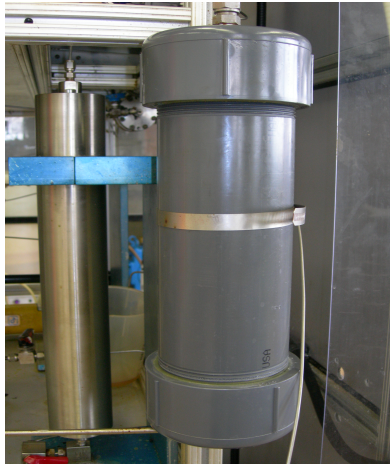
Figure 3.19 PVC refill tank
