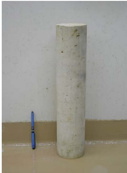
Figure 2.1 4 inch diameter 20 inch long core sample
