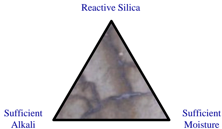
Figure 2.4 The Three Necessary Components for ASR-induced Damage in Concrete (Folliard et al, 2006).
