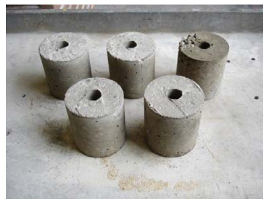
Concrete samples after demolding
