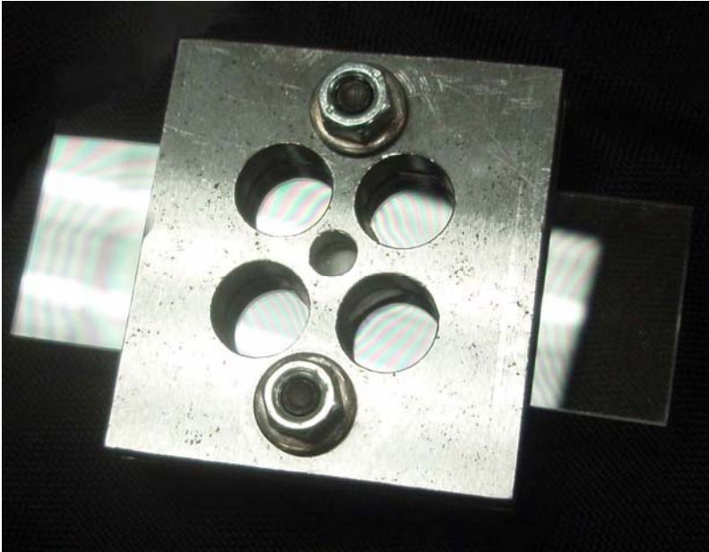
Figure 48: Testing of custom made new clamp for stressing the wafers
