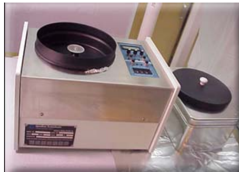
Figure 18: Spin coater (from website of Micro Chemical Facility, Texas A&M University)
