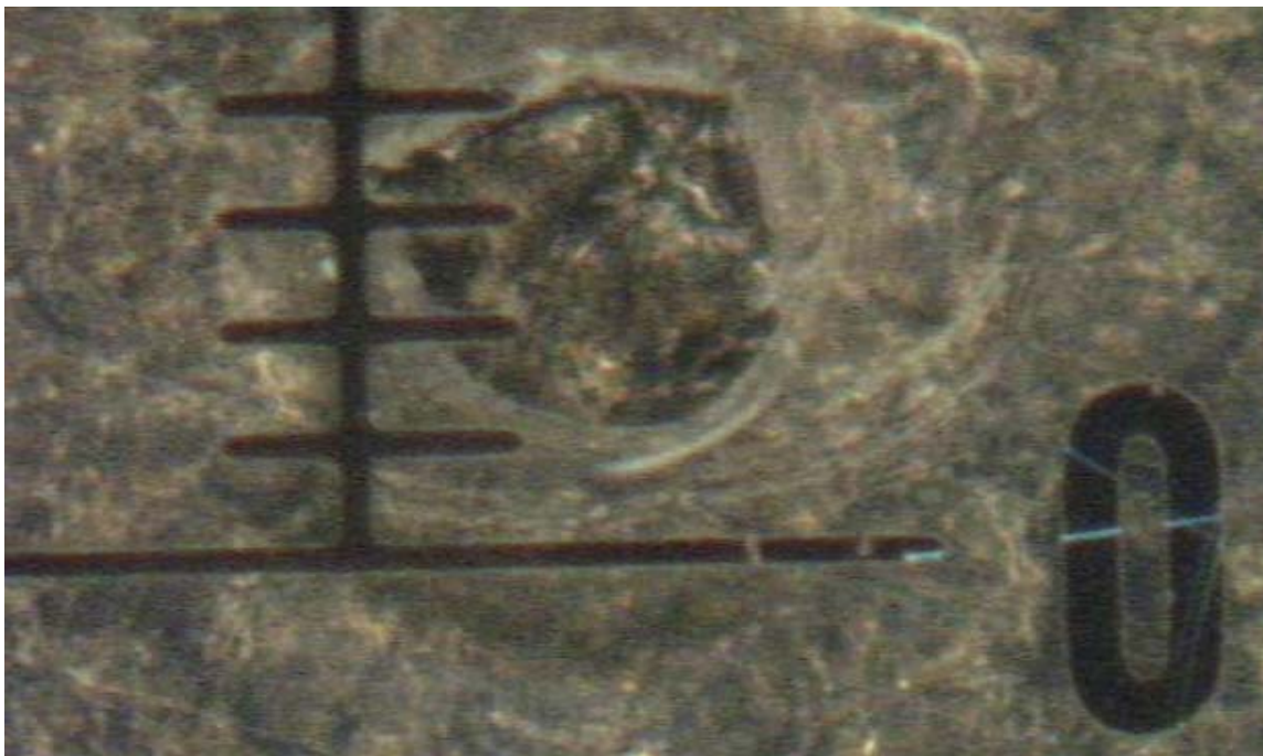
Figure 42: An aperture ( 75\mu\text{m} diameter) on a Teflon sheet
