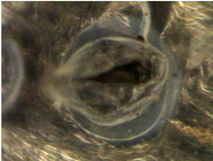
Figure 41: Extruded Teflon sheet during hot punching
