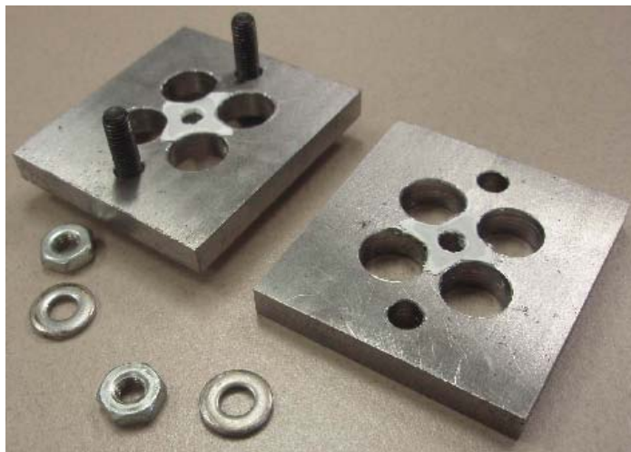
Figure 46: Custom made new clamp (exploded view)
