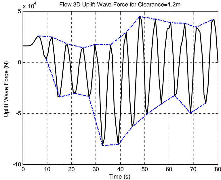
Figure 3.28: Flow3D uplift wave force for H=2m, T=6s, D=6m at clearance=1.2m
