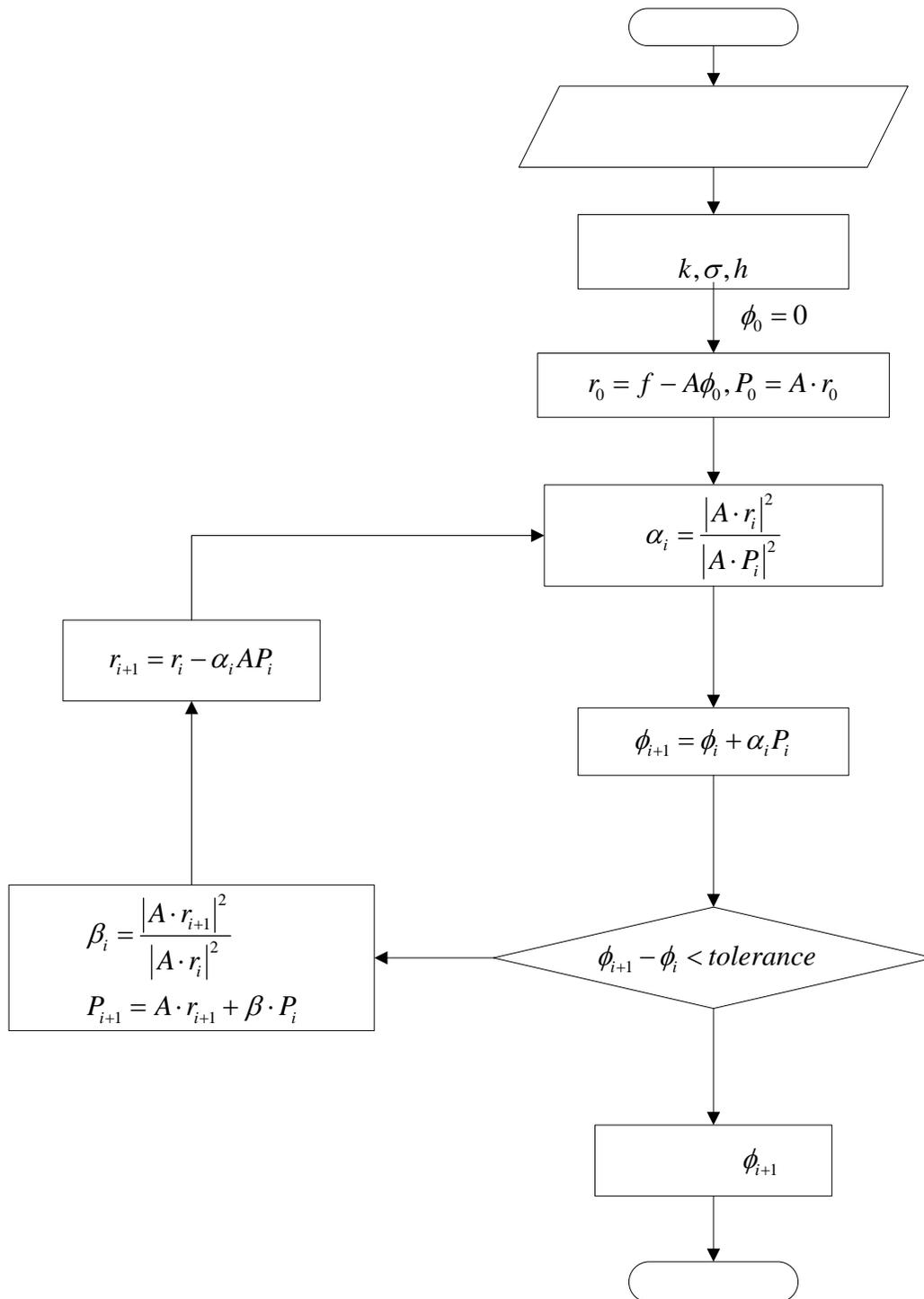
Figure 3.3: Flow chart of wave velocity potential calculation (Panchang et al., 1991)
