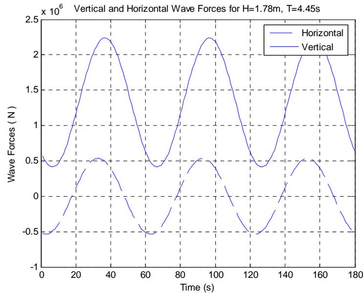
Figure 4.15: Wave force on bridge in reference model with  $H=1.78\text{m}$ ,  $T=4.45\text{s}$
