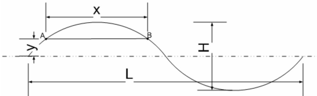
Figure 3.18: Sketch of incoming sinusoidal wave and clearance
