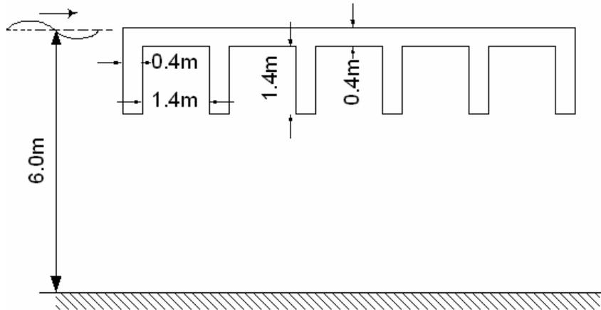
Figure 3.19: Geometry of the bridge deck and girders of reference model
