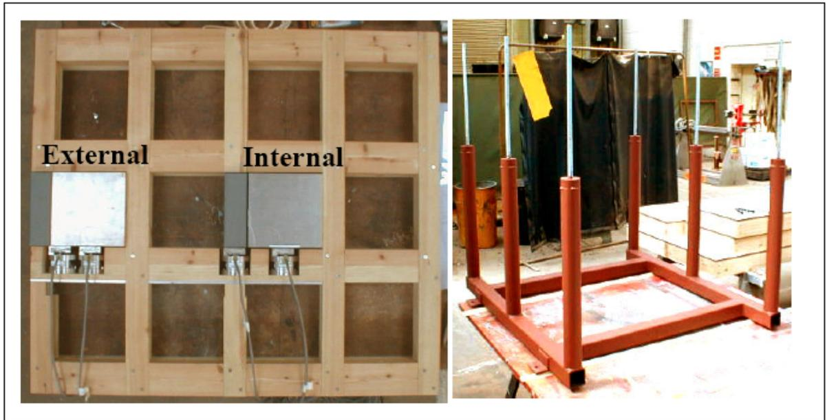
Figure 3.15: Down-standing frame of beams with testing elements and support pile structure (Tirindelli et al., 2002)
