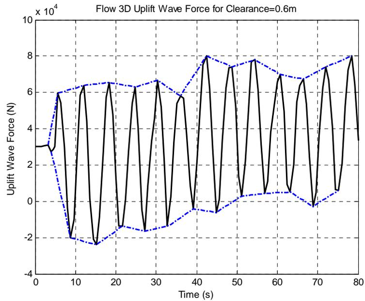
Figure 3.25: Flow3D uplift wave force for  $H=2\text{m}$ ,  $T=6\text{s}$ ,  $D=6\text{m}$  at clearance=0.6m
