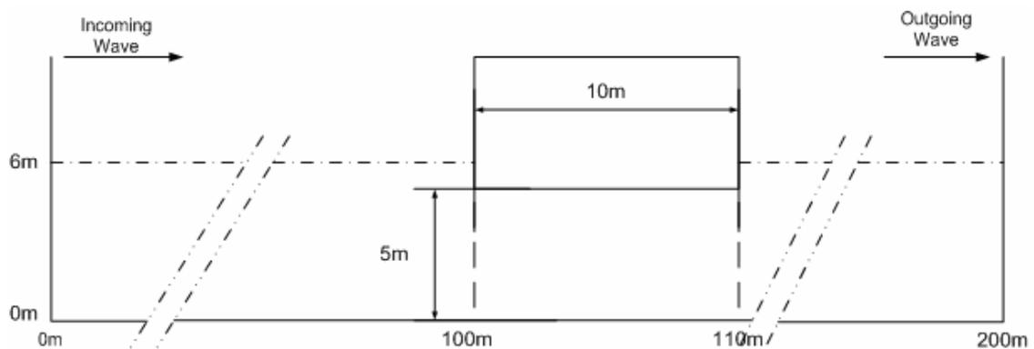
Figure 3.10: Model descriptions for comparison between Flow3D and 2D Model
