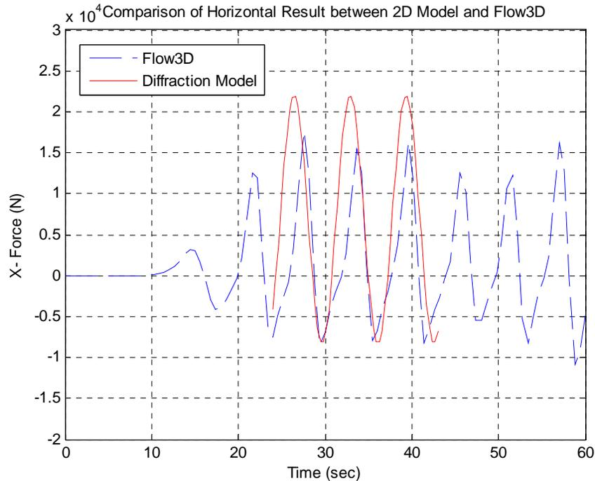
Figure 3.13: Comparison of horizontal wave force results between Flow3D and 2D Model
