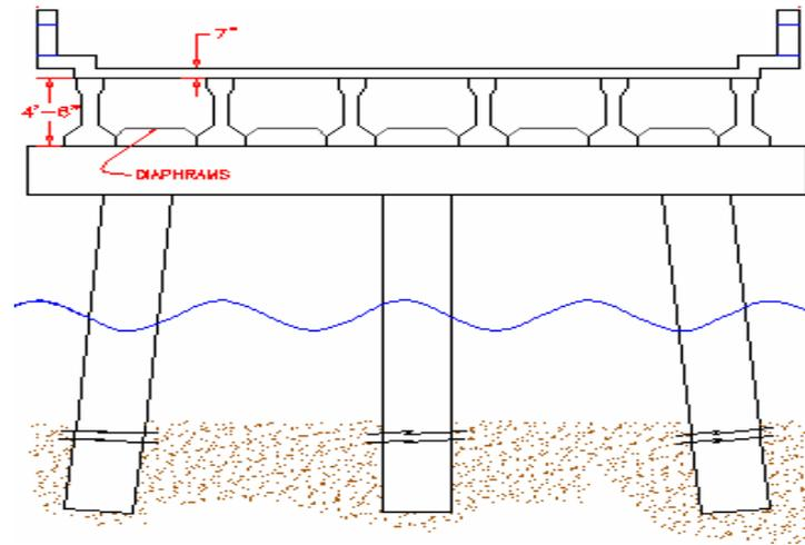
Figure 4.11: 2-D structural dimensions of I-10 Bridge over Escambia Bay
