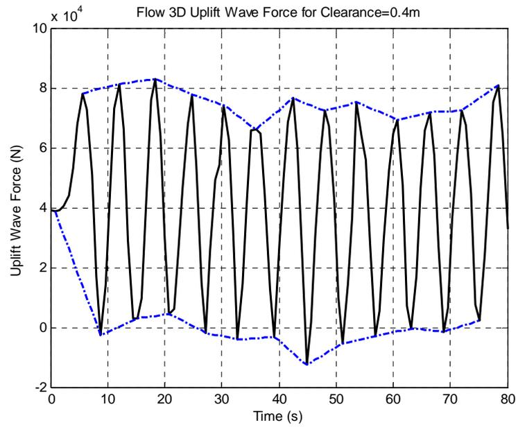
Figure 3.24: Flow3D uplift wave force for  $H=2\text{m}$ ,  $T=6\text{s}$ ,  $D=6\text{m}$  at clearance=0.4m
