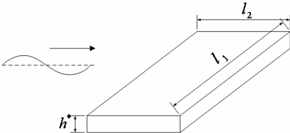
Figure 5.21: A figure showing the relative buoyancy height  $h^*$  (The cube in the figure has the same volume as the model bridge)
