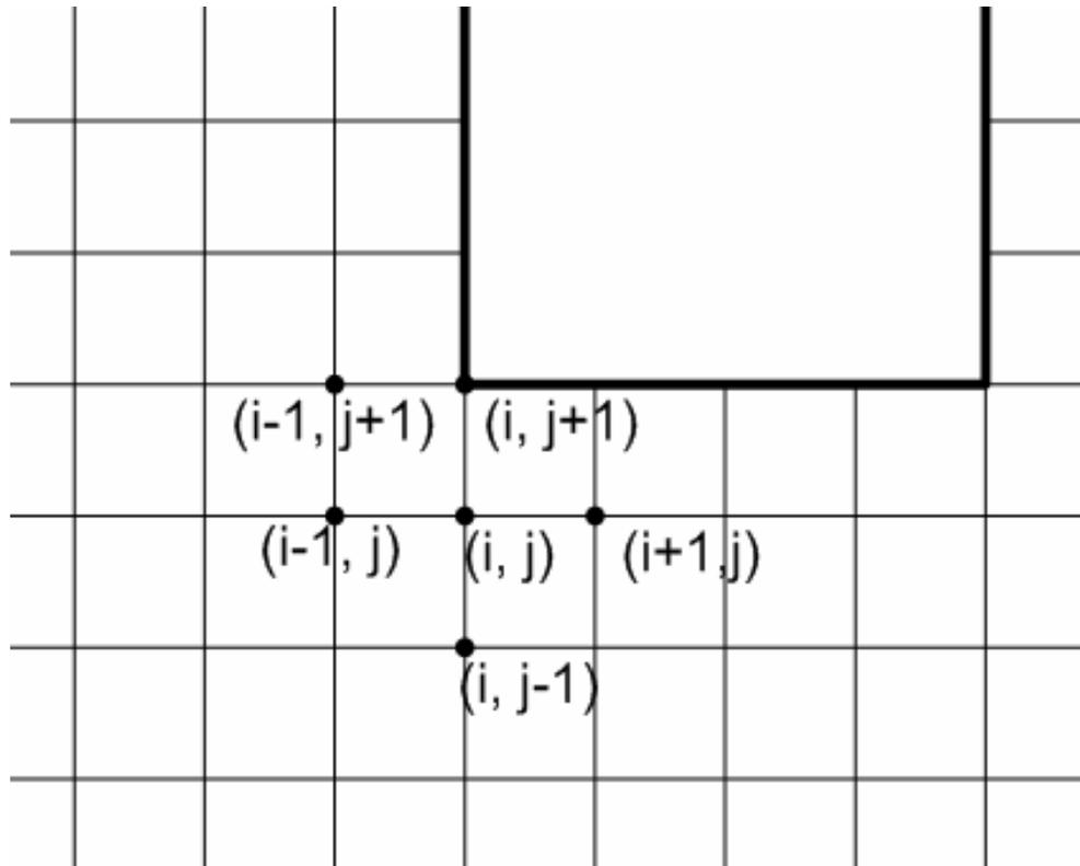
Figure 3.2: Calculation domain grids around a corner of structure
