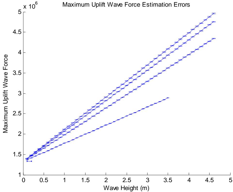
Figure 5.23: Maximum uplift wave force estimation errors for wave periods of 2s, 4s, 6s, 8s and 10s
