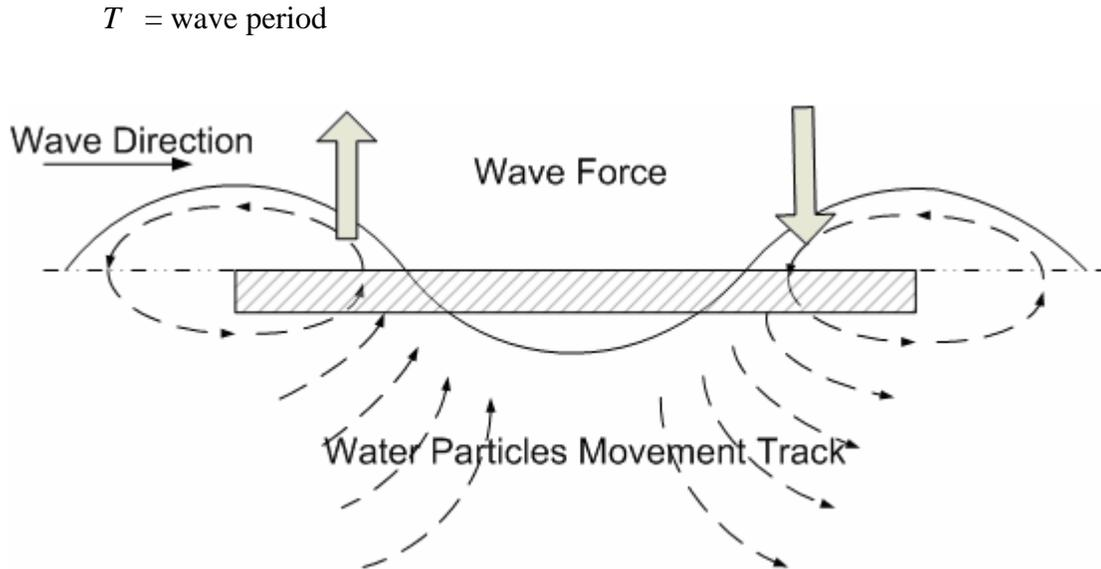
Figure 5.20: General view of bridge in waves
