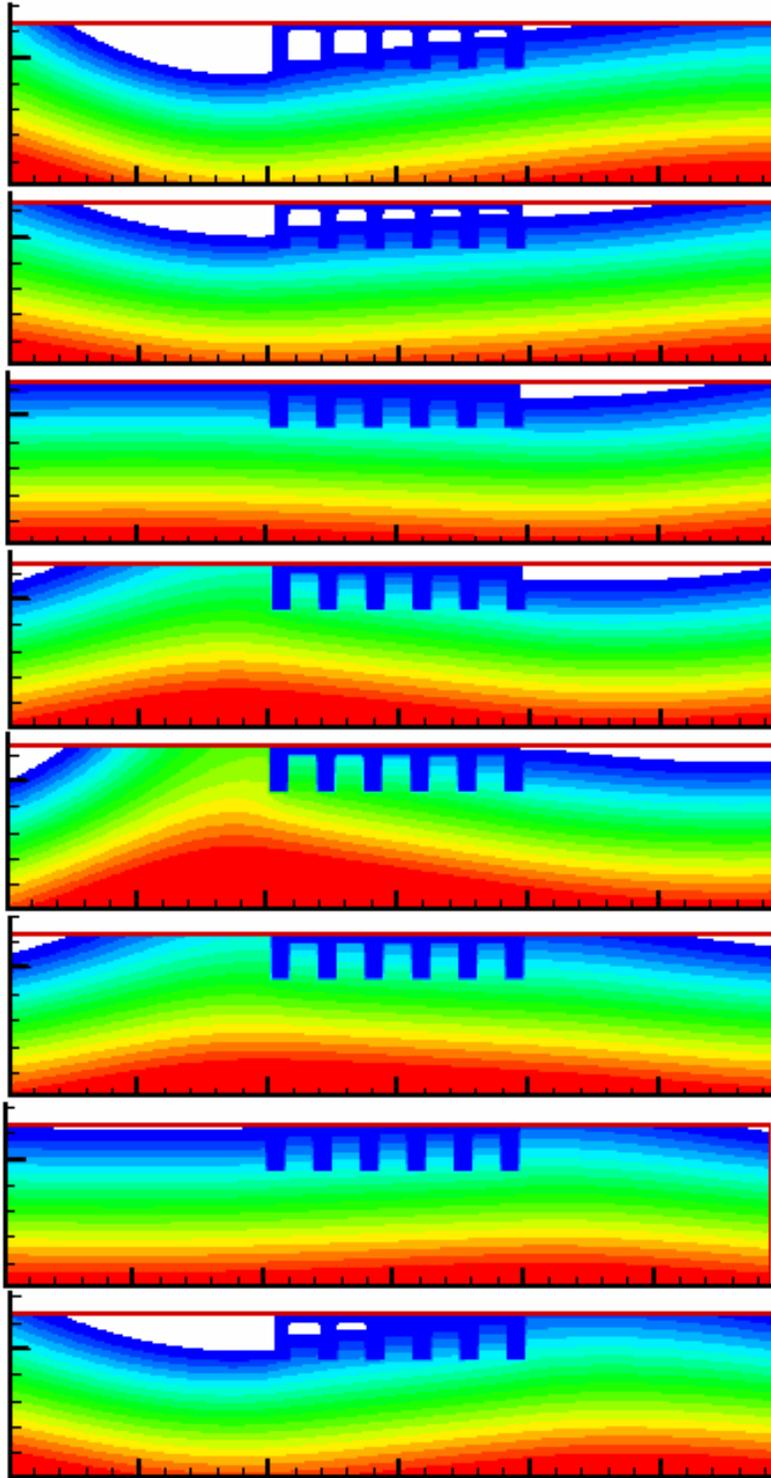
Figure 4.14: Calculation domain pressure contour as waves pass by
