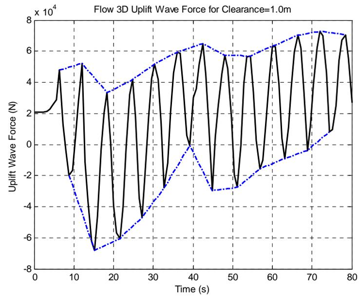
Figure 3.27: Flow3D uplift wave force for H=2m, T=6s, D=6m at clearance=1.0m
