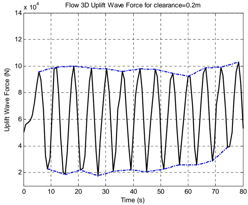
Figure 3.23: Flow3D uplift wave force for H=2m, T=6s, D=6m at clearance=0.2m
