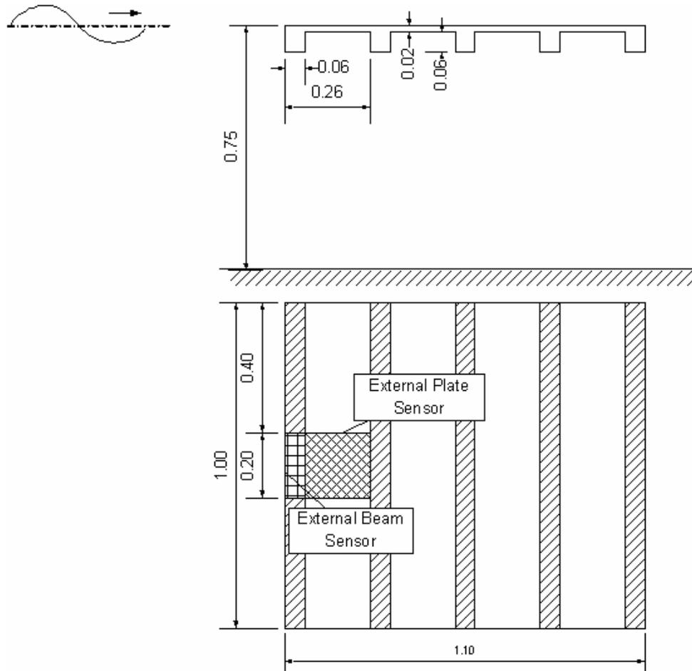
Figure 3.17: 2D wave velocity potential model (metric unit)
