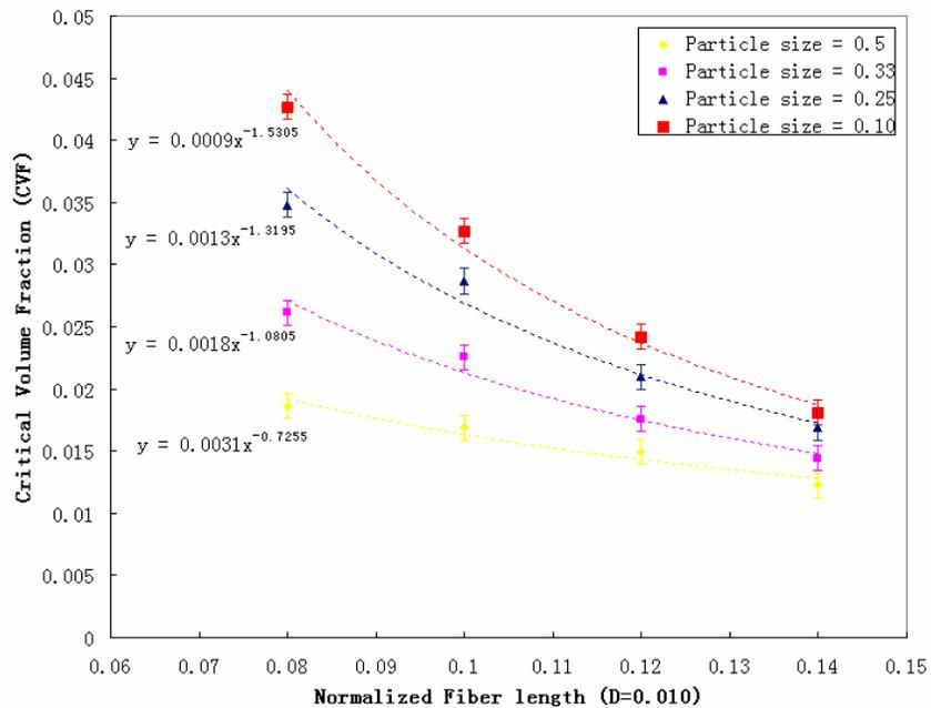
Fig. 18. Normalized fiber length vs. critical volume fraction of samples with emulsion particles ( $D = 0.010$ )
