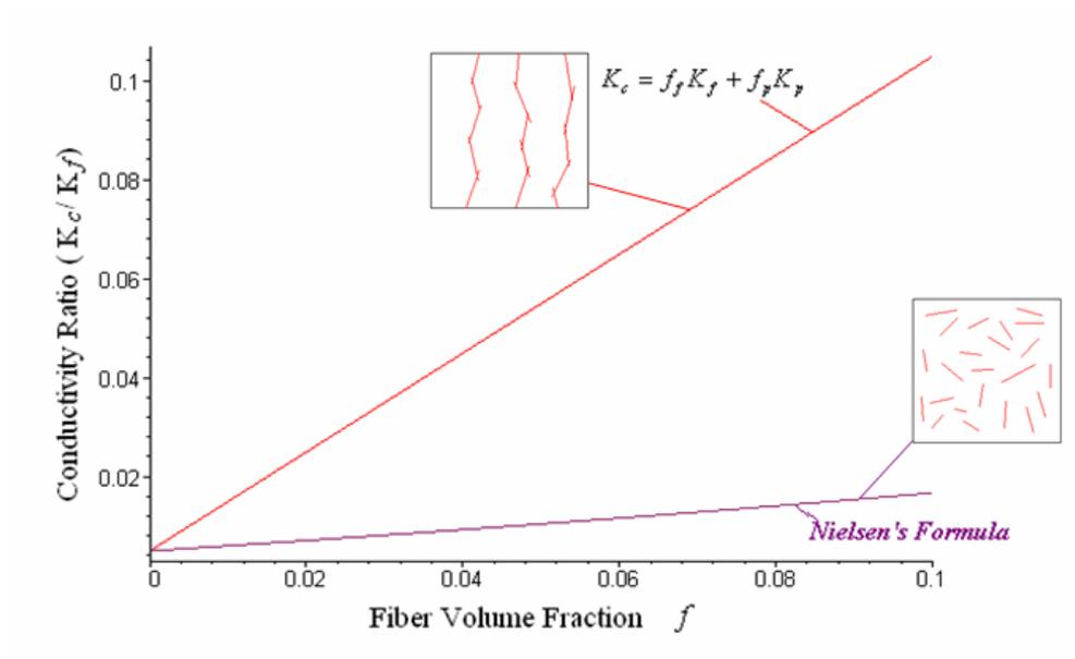
Fig. 22. Plotting of two thermal conductivity equations
