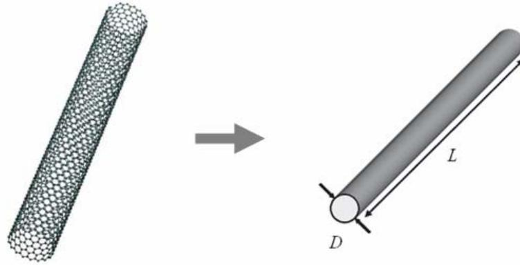
Fig. 3. Equivalent continuum model of carbon nanotubes
