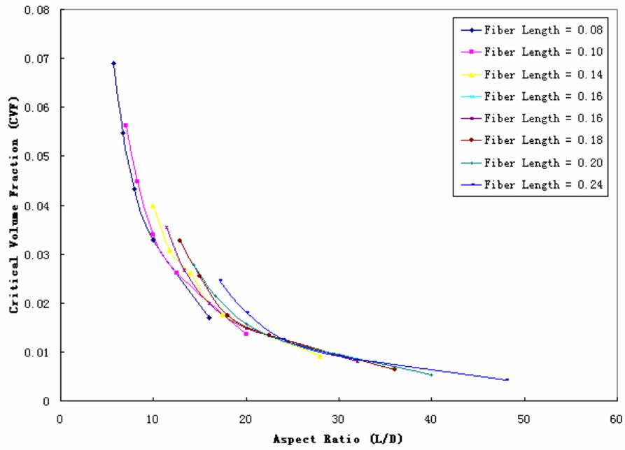
Fig. 12. Critical volume fraction vs. aspect ratio
