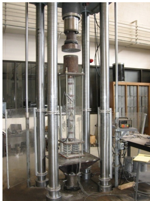
Figure 4.10. Loading with 500 kip (2220 kN) MTS Machine.
