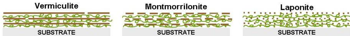
Figure 45. Schematic images of the nanostructure of clay-based assemblies made with platelets of varying diameters. Each clay-polymer bilayer could be 1 – 30 nm thick depending on deposition conditions.
