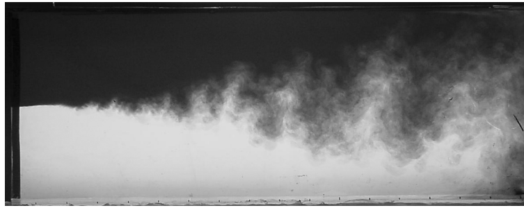
Figure 2.2 Photographic image of a hot/cold water experiment in the water channel. The mean flow is from left-to-right.
