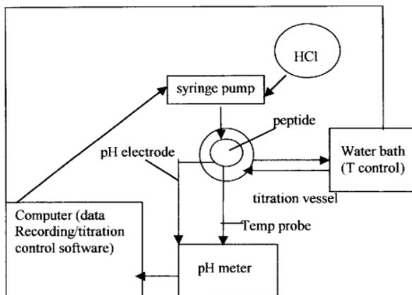
Figure 3: Apparatus for titration of model peptides. The syringe pumps HCl into the titration vessel, using volume and time increments programmed into the computer. From the pH meter and temperature probe, the computer records the pH and temperature of the titration vessel, respectively, at each point. The water bath keeps the titration vessel at  $25 \pm 1^\circ\text{C}$ .
