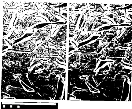
Figure 27. SEM stereo photographs of representative area of the advanced stage of dissolution interval III. Microtopography consists of etched cracks (A), polygonal widened cracks (B), and v-shaped notches (C). Scale bar equals 100 \mu\text{m} .
