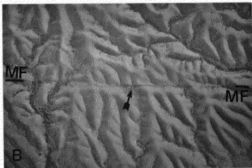
Figure 4. A) Low-sun-angle aerial photograph of the Pointer Site "X" (fault trace between line segments labeled "MF"). B) Low-sun-angle of the alluvial fan site.
