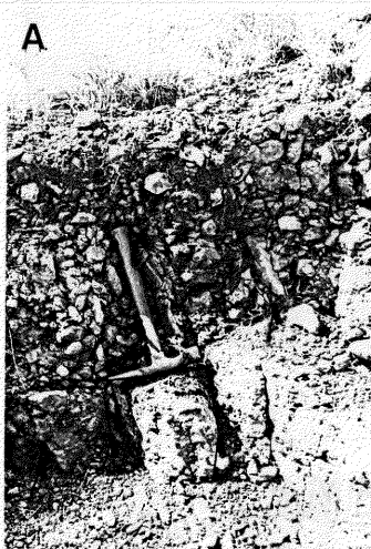
Figure 18. A) The vertical sandstone dikes (arrows) in the bedrock pit site (parallel to hammer handle). B) One of the two thin horizontal sandstone laminations seen on the up-block (arrows) in the bedrock pit site.
