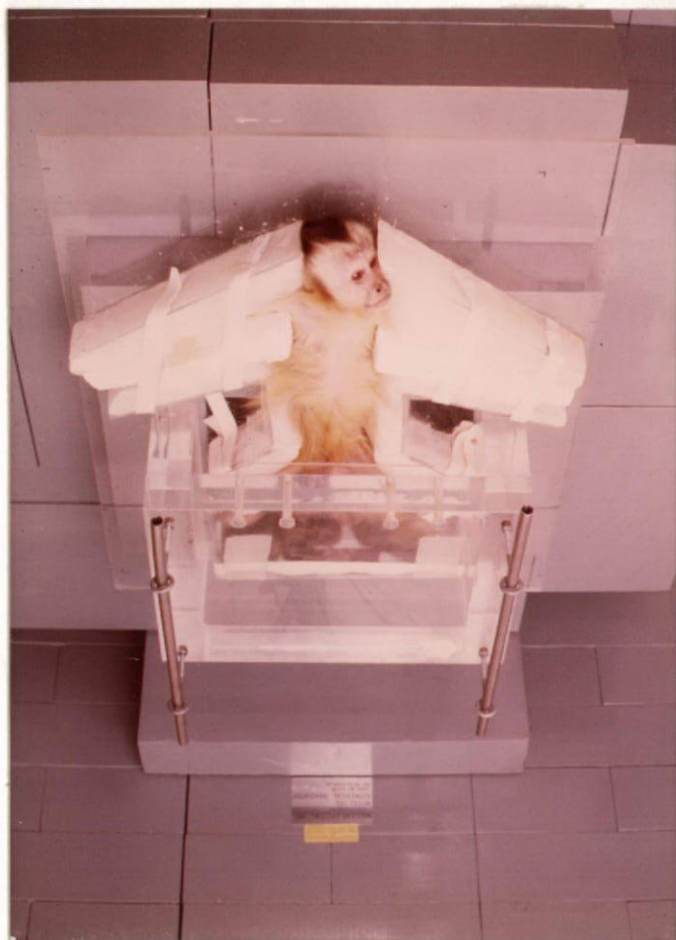
FIGURE 3 Photograph of the monkey in holder for leg irradiation. Here shown with a plexiglass instead of a paraffin moderator.
