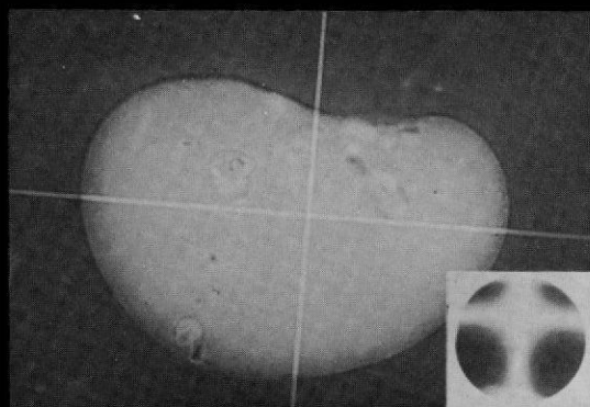
Well rounded grain of tourmaline from sample 2-8. Insert shows uniaxial interference figure obtained from this grain. Transmitted light, n=1.66 , X225.
