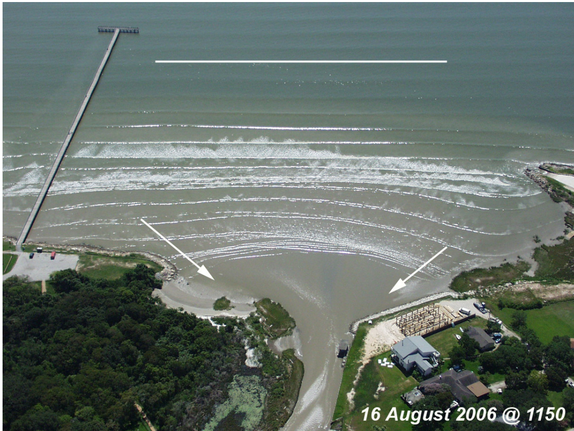
Figure 25. White line shows incoming waves are parallel offshore, then as the wave train approaches the sand bar the waves “feel bottom” and refract around the sand bar. Every train of ship waves brings in more sand to Pine Gully in this way.
