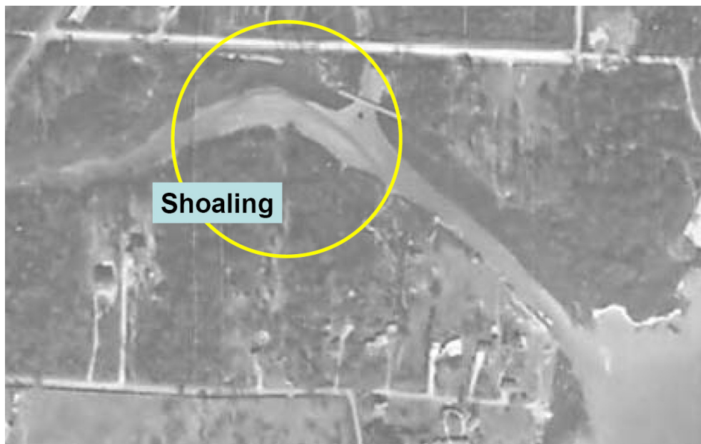
Figure 35. 1986 aerial photograph of Pine Gully report given to the City of Seabrook by Dr. Sherman. Figure is pulled directly out of presentation.
