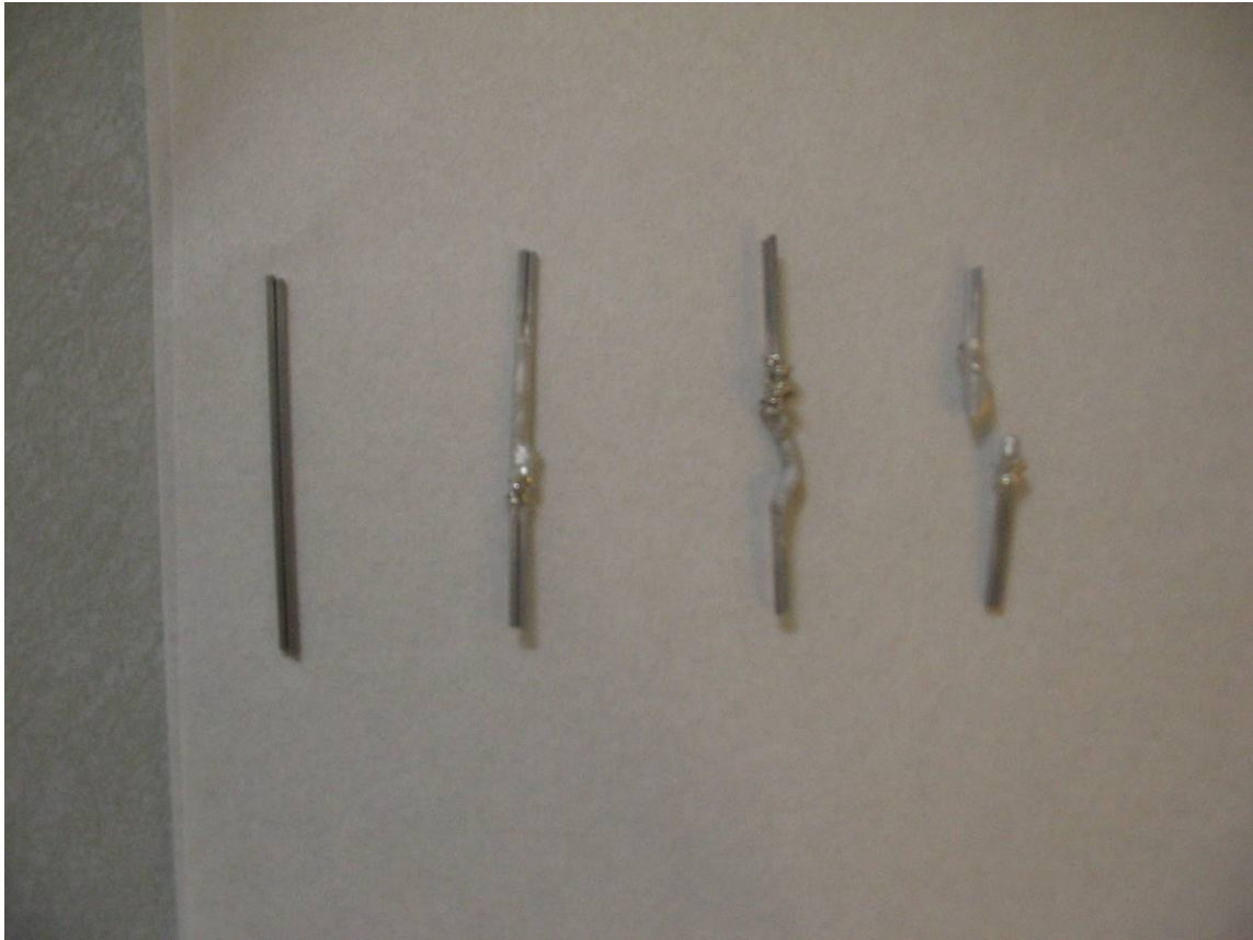
Fig. 2.25 Sources Used for Deposition. (Left from Right: Bare Tungsten Bars before Use, Used Alumel Source and Two Used Chromel Sources.)
