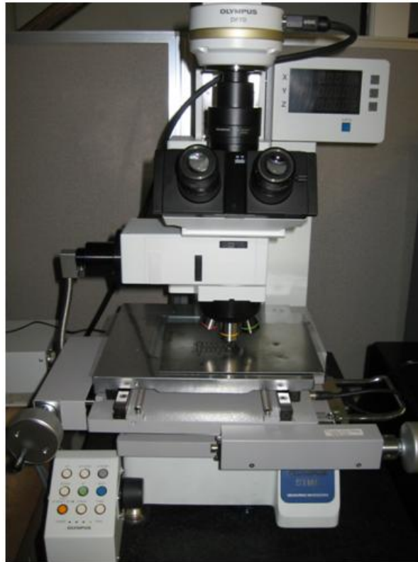
Fig. 3.1 Optical microscope used for measuring the geometry of indentation
