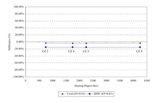
Figure 6.87 Percent difference of annual energy use (base case (0.55 EF) vs. 0.65 EF)
