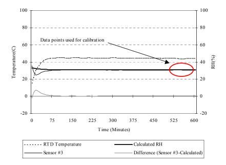
Figure A.41 Time series and residual plot of sensor #3 and calculated RH for Magnesium Chloride before calibration
