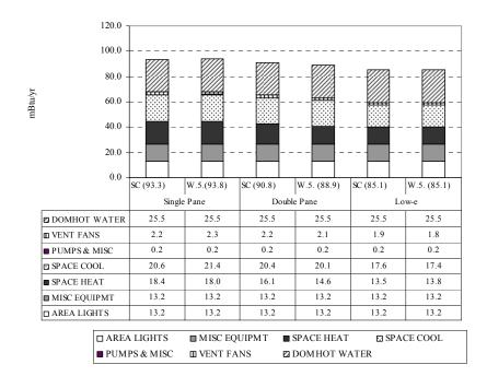
Figure 6.11 Annual building energy performance report using the thermal mass mode
