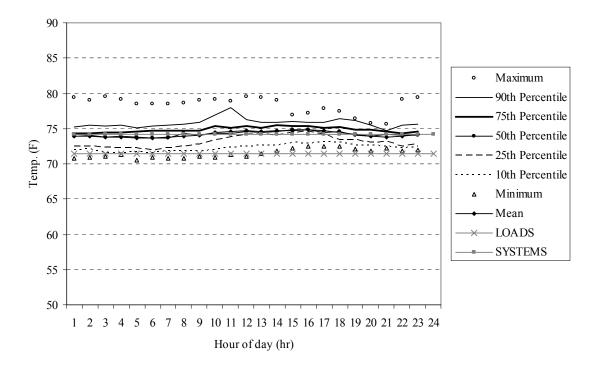
Figure 5.28 Indoor temperature profile for the period August 1 to August 14, 2004
