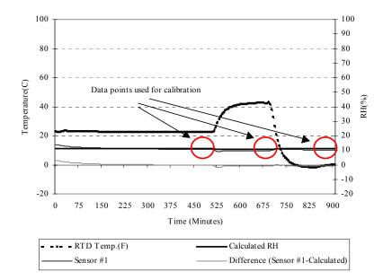
Figure A.28 Time series and residual plot of sensor #1 and calculated RH for Lithium Chloride before calibration
