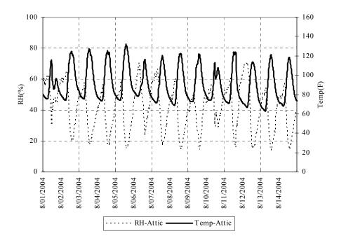
Figure 4.31 Attic relative humidity and temperature (CH3811, CH3812)
