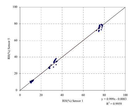
Figure A.46 Comparison plot of sensor #5 vs. sensor #1
