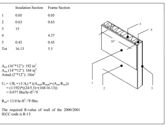
Figure 4.75 Wood frame wall dimension and calculated R-value
