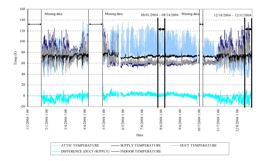
Figure 5.25 Measured attic, supply and duct temperature, and difference between duct and supply temperature
