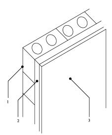
Figure 4.78 8" concrete block wall with perlite and concrete fill
