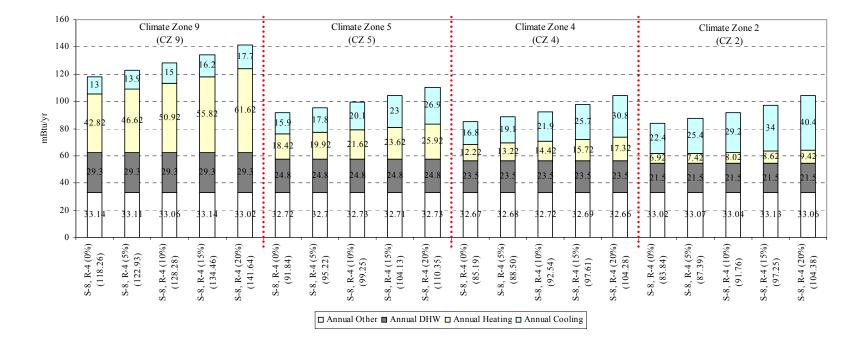
Figure 6.45 Annual energy use of SR-8 and RR-4 according to the duct leakage rate
