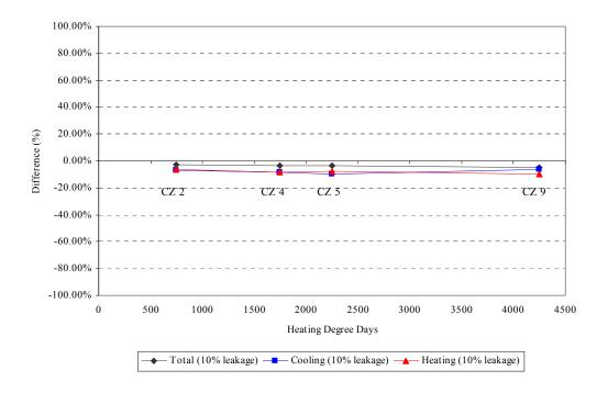
Figure 6.94 Percent difference according to HVAC location (the attic space vs. the conditioned space (10% duct leakage rate))
