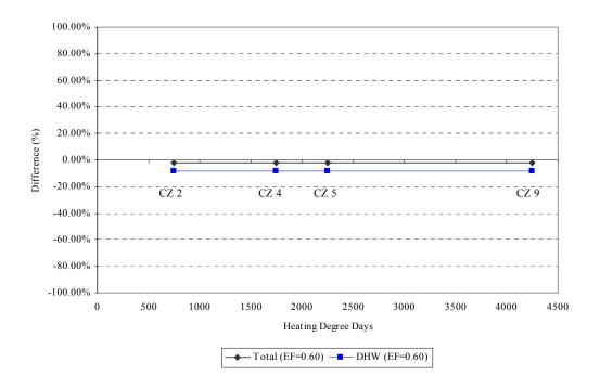
Figure 6.86 Percent difference of annual energy use (base case (0.55 EF) vs. 0.60 EF)
