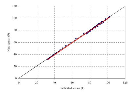
Figure A.26 Comparison of new sensor #5 against calibrated sensor #1
