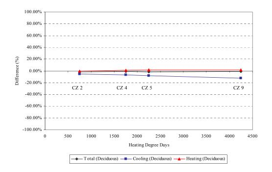
Figure 6.107 Percent difference of annual energy use (base case (no shading) vs. both (east and west) side shading of deciduous))
