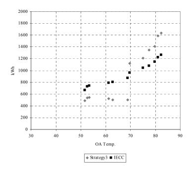
Figure 5.11 Comparison between the IECC and strategy #3 of electricity
