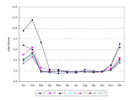
Figure 5.69 Monthly natural gas use from the measured data of the case-study house and DOE-2 simulations
