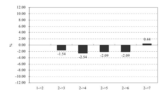
Figure 6.3 Annual energy consumption difference between thermal mass modes
