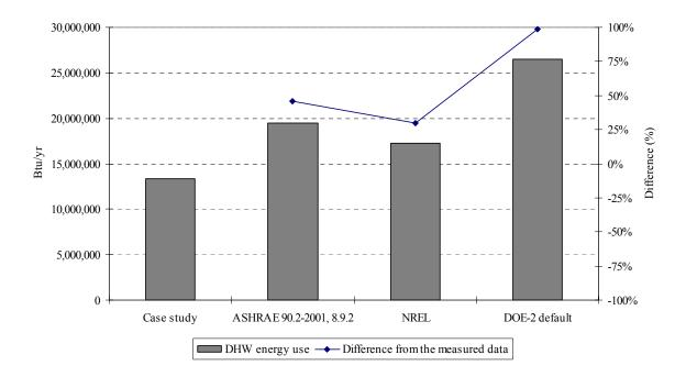
Figure 5.63 Comparison of DHW energy use (pilot light = 900 Btu/hr)
