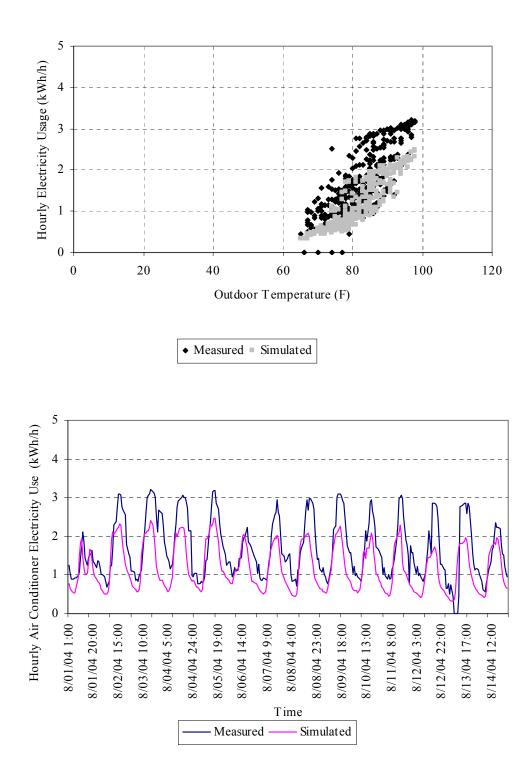
Figure 5.51 Cooling energy plots without duct model for two weeks (08/01/2004 – 08/14/2004)
