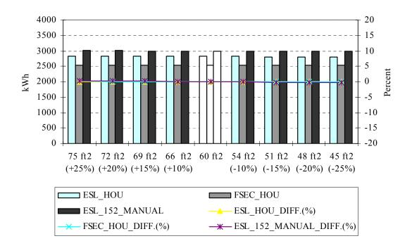
Figure I.2 The variation of return duct area and results
