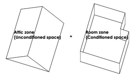
Figure 4.47 Zones of the as-built base-case house
