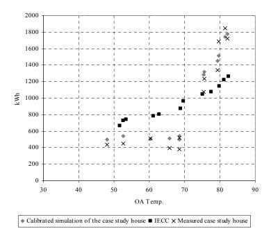
Figure 5.5 Measurement and calibration results of the electricity
