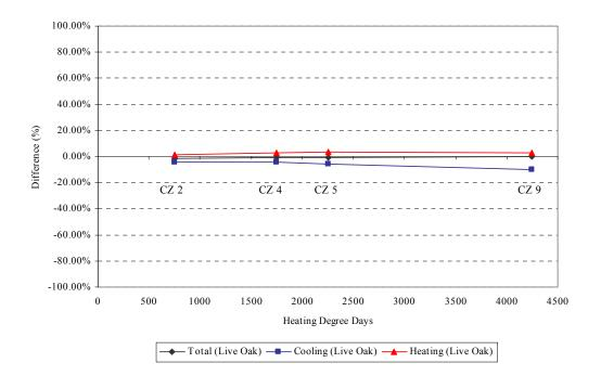
Figure 6.98 Percent difference of annual energy use (base case (no shading) vs. east side shading of live oak))
