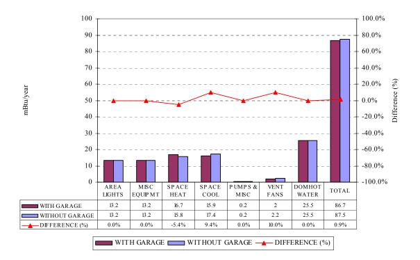
Figure J.2 Comparison results with and without garage space
