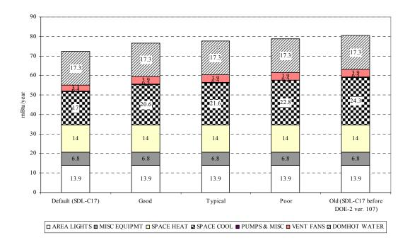
Figure 5.60 BEPS results according to the different A/C curves
