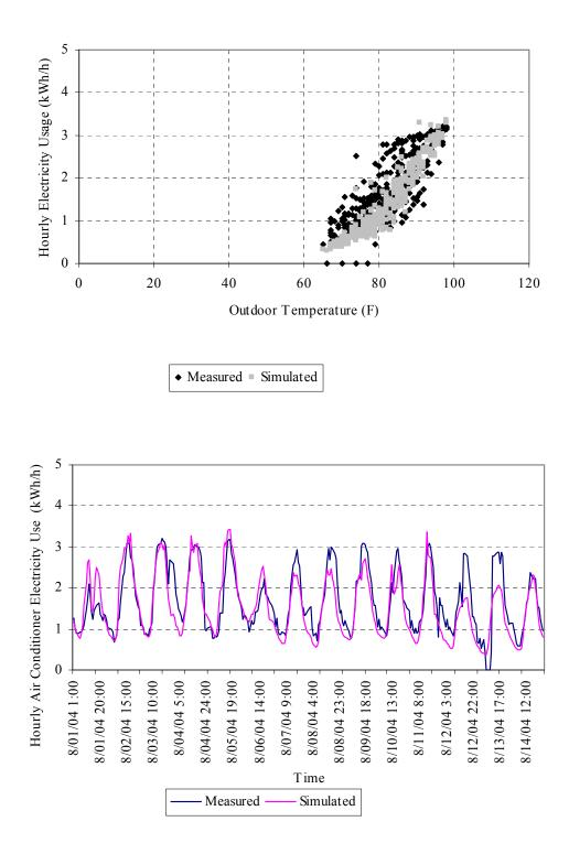
Figure 5.54 Cooling energy with default A/C curve (new SDL-C17)
