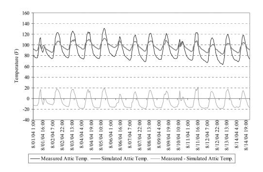
Figure 5.40 The uncalibrated simulation (run #1) and measured results of the attic temperature for the period August 1 to August 14, 2004
