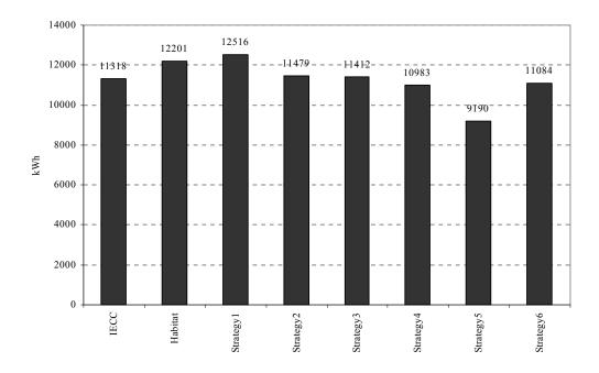
Figure 5.19 One-year electricity use of each simulation
