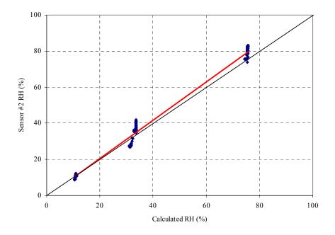
Figure A.37 Comparison of sensor #2 against calculated RH before calibration
