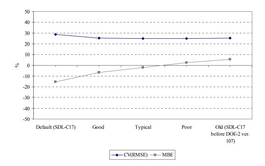
Figure 5.59 CV (RMSE) and MBE according to the different A/C curves
