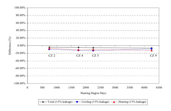
Figure 6.95 Percent difference according to HVAC location (the attic space vs. the conditioned space (15% duct leakage rate))
