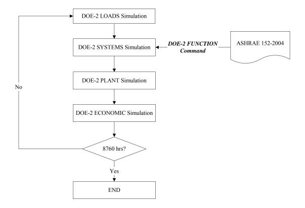
Figure 4.66 DOE-2 input function method for ASHRAE 152-2004
