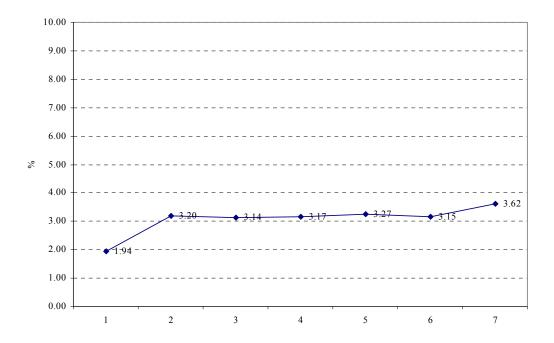
Figure 6.8 Total energy difference between with thermostat setback and without thermostat setback
