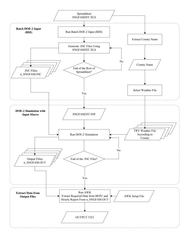
Figure 4.67 Procedure for using the BDI
