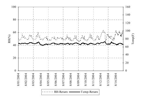
Figure 4.30 Return relative humidity and temperature (CH3803, CH3804)
