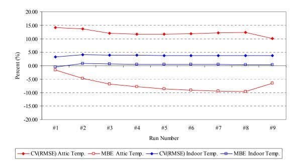
Figure 5.49 CV(RMSE) and MBE of attic and indoor temperature calibration
