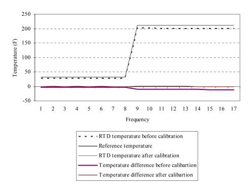
Figure A.4 Residual plot of the RTD sensor against reference temperature
