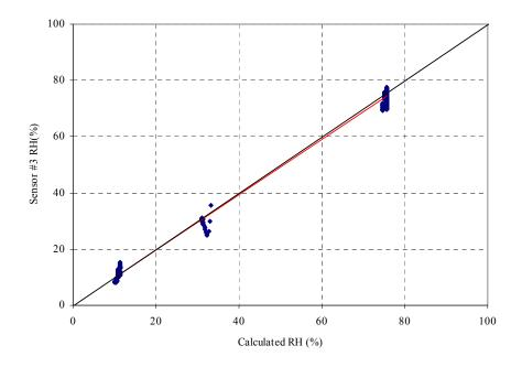
Figure A.43 Comparison of sensor #3 against calculated RH before calibration
