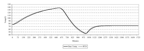
Figure A.69 Time series plot of duct sensor vs. RTD sensor
