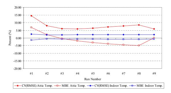
Figure 5.44 CV(RMSE) and MBE of attic and indoor temperature calibration
