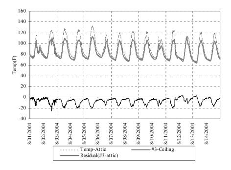
Figure 4.37 Ceiling surface temperature in the attic
