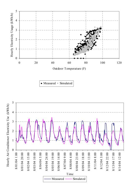
Figure 5.53 Cooling energy plots with duct model for two weeks (08/01/2004 – 08/14/2004)
