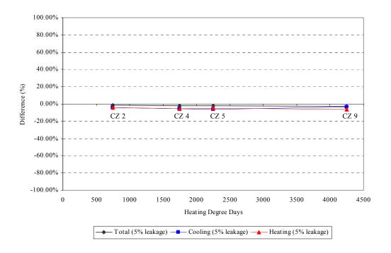
Figure 6.93 Percent difference according to HVAC location (the attic space vs. the conditioned space (5% duct leakage rate))
