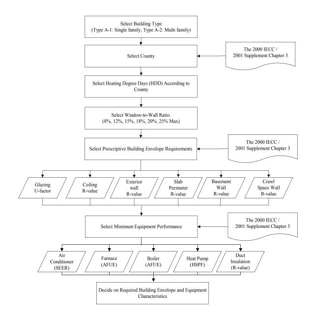
Figure 4.61 Procedure to determine the building envelope and equipment characteristics
