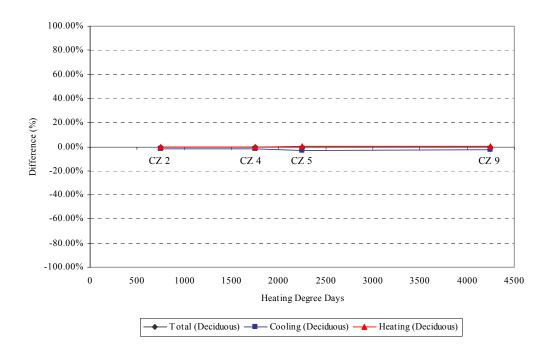
Figure 6.103 Percent difference of annual energy use (base case (no shading) vs. west side shading of deciduous))
