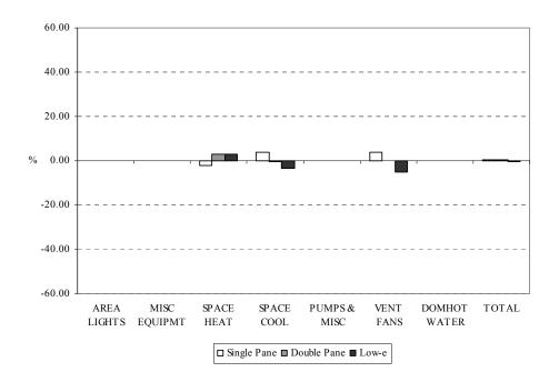
Figure 6.10 Percentage difference between SC and W-5 using the quick mode
