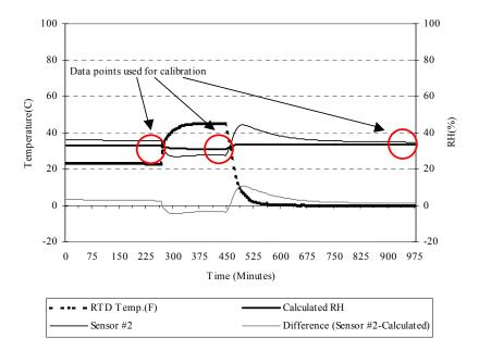
Figure A.35 Time series and residual plot of sensor #2 and calculated RH for Magnesium Chloride before calibration
