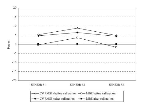
Figure A.48 CV(RMSE) and MBE plot before and after calibration
