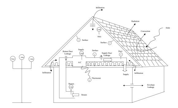
Figure 4.6 Diagram of sensor location
