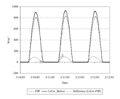
Figure A.60 PSP and Li-Cor time series plot before calibration.
