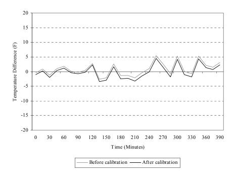
Figure A.58 Residual plot before and after calibration.
