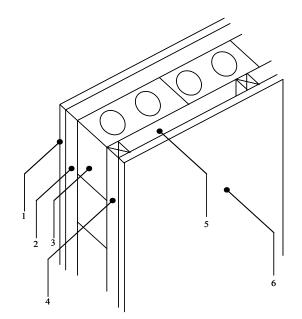
Figure 4.80 8" concrete block wall with perlite and concrete filled
