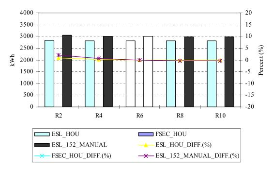
Figure I.4 The variation of return duct R-value and results
