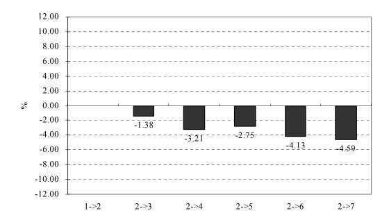
Figure 6.4 Cooling energy consumption difference between thermal mass modes
