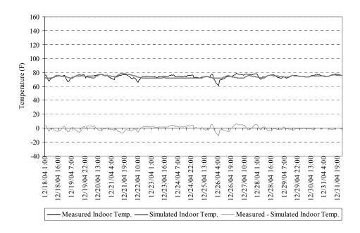
Figure 5.46 The uncalibrated simulation (run #1) and measured results of the indoor temperature for the period December 18 to December 31, 2004
