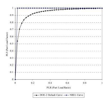
Figure 4.57 Domestic hot water efficiency curves for the DOE-2 program (NREL 2001)
