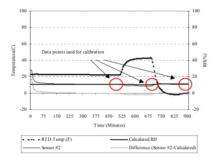
Figure A.34 Time series and residual plot of sensor #2 and calculated RH for Lithium Chloride before calibration
