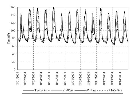
Figure 4.34 Attic temperature and roof surface temperatures
