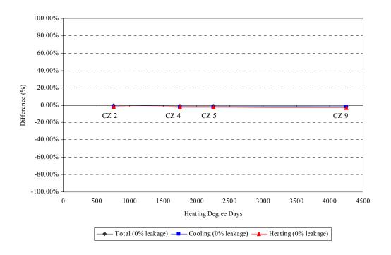
Figure 6.92 Percent difference according to HVAC location (the attic space vs. the conditioned space (0% duct leakage rate))
