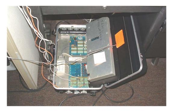
Figure A.1 Synergistics portable data logger (C180-XP) used for the calibration procedure
