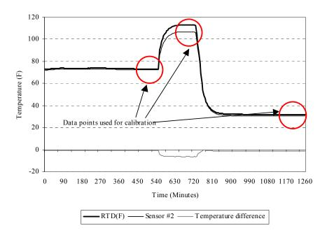
Figure A.10 Time series and residual plot of the RTD sensor and sensor #2 before calibration
