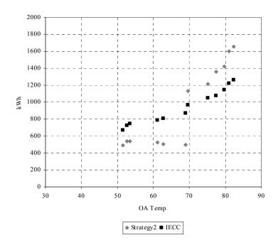
Figure 5.9 Comparison between the IECC and strategy #2 of electricity
