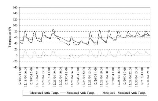
Figure 5.45 The uncalibrated simulation (run #1) and measured results of the attic temperature for the period December 18 to December 31, 2004
