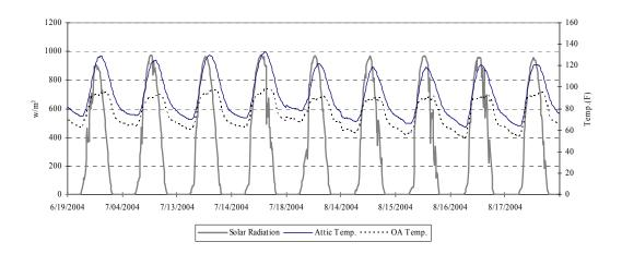
Figure 5.37 Measured solar radiation, attic and OA temperature on clear days
