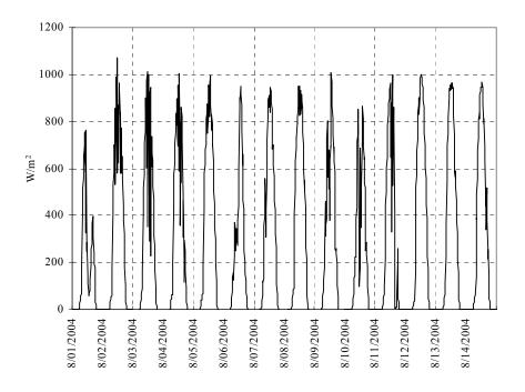
Figure 4.41 Global horizontal solar radiation (CH3807)
