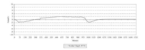
Figure A.68 Residual plot between supply and RTD sensor
