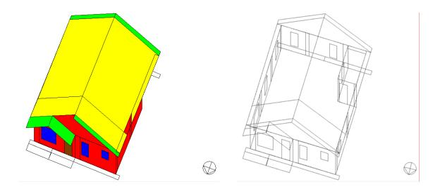
Figure 4.51 Image of the as-built case-study house simulation input using the DrawBDL program
