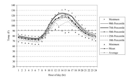
Figure 5.30 Attic temperature profile for the period August 1 to August 14, 2004
