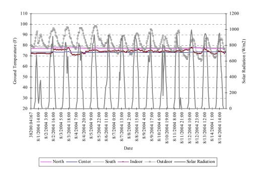
Figure 5.64 Three ground temperatures versus solar radiation for summer period
