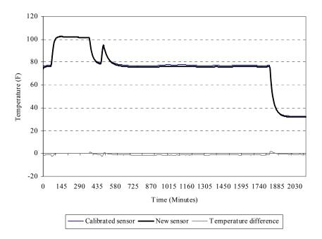
Figure A.25 Time series plot of new sensor #5 and calibrated sensor#1
