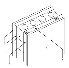
Figure 4.79 8" concrete block wall with perlite fill
