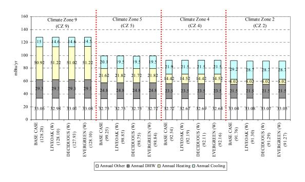
Figure 6.105 Annual energy use of west side tree shading
