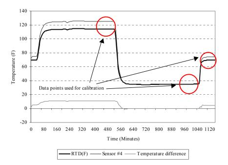
Figure A.20 Time series and residual plot of the RTD sensor and sensor #4 before calibration
