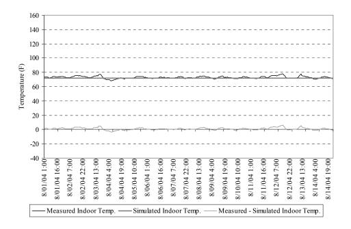
Figure 5.41 The uncalibrated simulation (run #1) and measured results of the indoor temperature for the period August 1 to August 14, 2004
