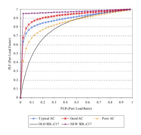
Figure 4.55 AC system curves for DOE-2 program (Henderson et al. 2000)
