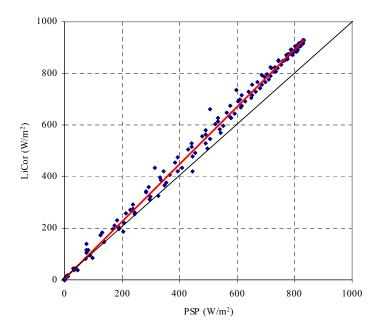
Figure A.61 PSP versus Li-Cor before calibration.
