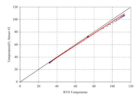
Figure A.11 Comparison of sensor #2 against RTD temperature before calibration
