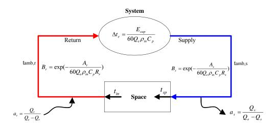
Figure 4.52 Schematic diagram of duct model (ASHRAE 152-2004)
