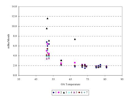
Figure 5.70 Monthly natural gas use from the measured data of the case-study house and DOE-2 simulations vs. average monthly outdoor temperature
