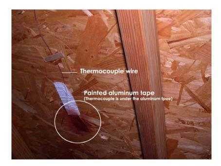
Figure 4.13 J-type thermocouple for measuring surface temperature of roof
