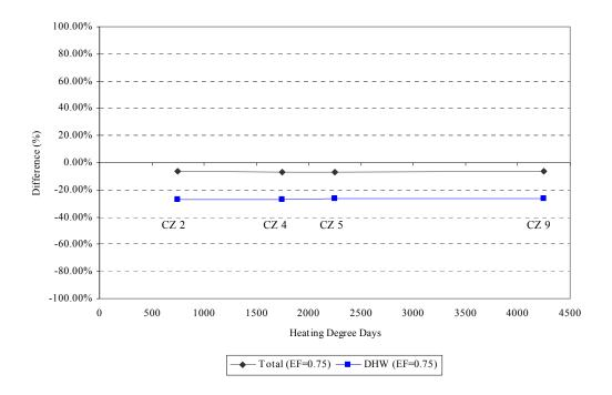
Figure 6.89 Percent difference of annual energy use (base case (0.55 EF) vs. 0.75 EF)
