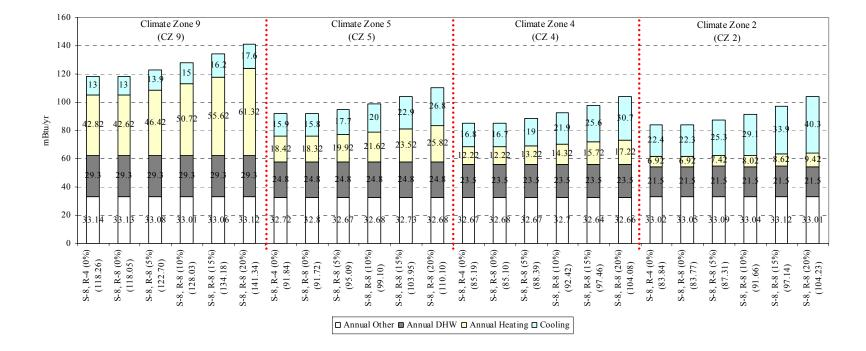
Figure 6.57 Annual energy use of SR-8 and RR-8 vs. SR-8 and RR-4 according to the duct leakage rate
