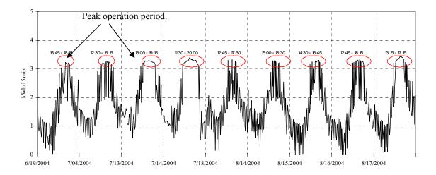
Figure 5.38 Measured AC and AC blower electricity (AC + AC blower) use
