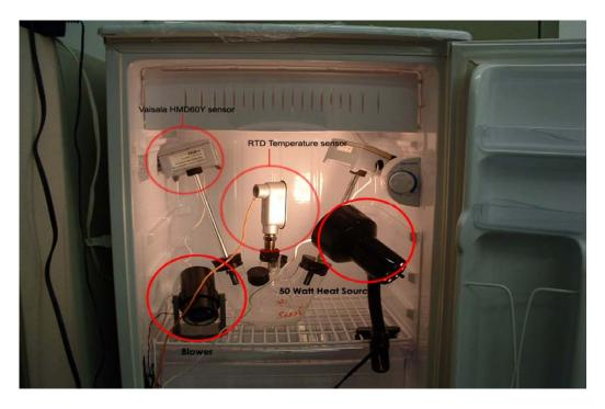
Figure A.2 Experimental setting showing the Vaisala and RTD sensors
