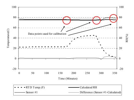
Figure A.30 Time series and residual plot of sensor #1 and calculated RH for Sodium Chloride before calibration
