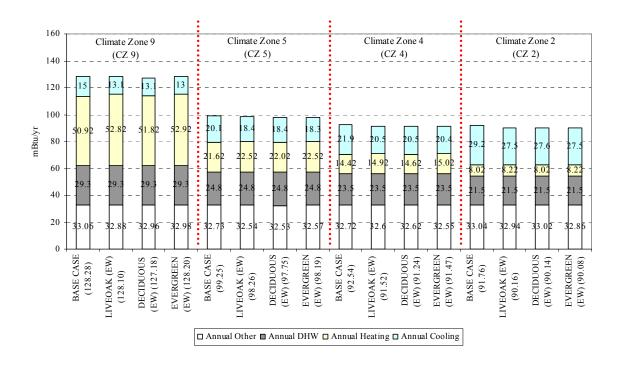
Figure 6.109 Annual energy use of both (east and west) side tree shading
