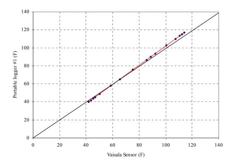
Figure A.50 Comparison of portable data logger #1 and Vaisala sensor before calibration.
