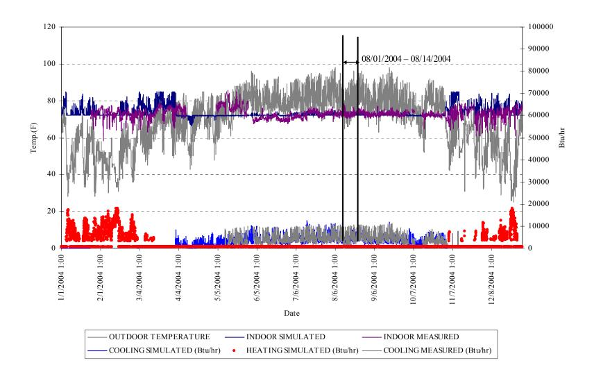
Figure 5.52 Temperature and cooling energy plots with duct model for whole year
