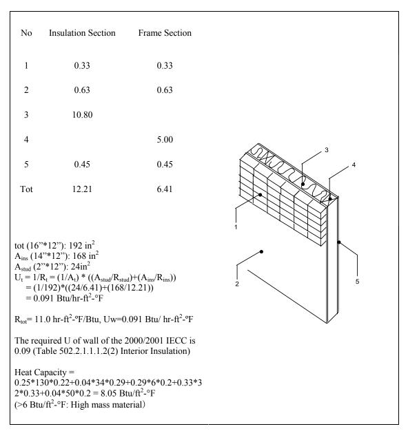
Figure 4.76 Facia brick wall dimension and calculated R-Value
