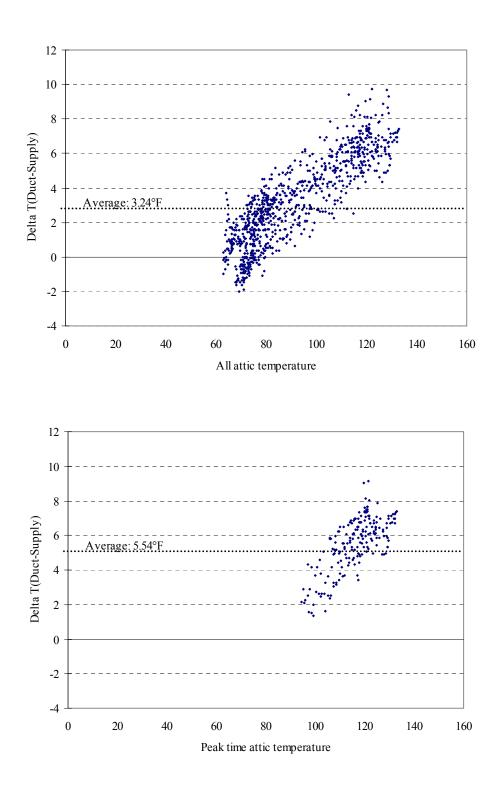
Figure 5.39 Plots of measured attic temp. vs. the difference between duct and supply temperatures
