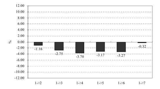
Figure 6.7 Annual energy consumption difference between quick mode and thermal mass modes without the thermostat setback
