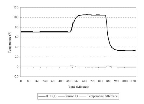
Figure A.17 Time series and residual plot of the RTD sensor and sensor #3 after calibration
