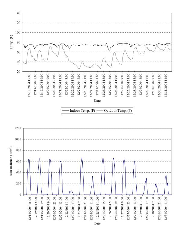
Figure 5.31 The indoor, outdoor temperature and solar radiation for the period December 18 to December 31, 2004
