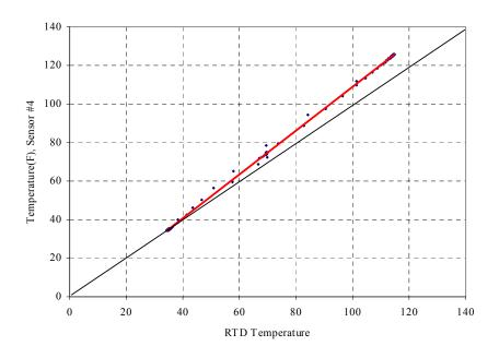
Figure A.21 Comparison of sensor #4 against RTD temperature before calibration
