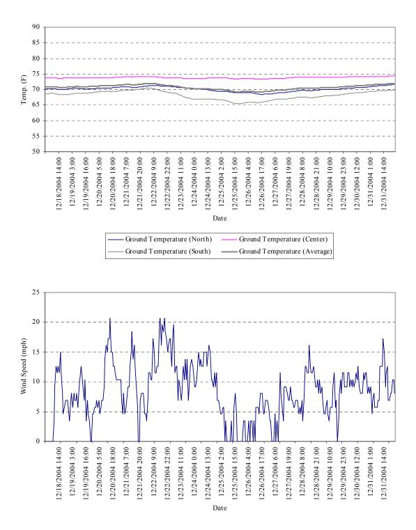
Figure 5.32 The ground temperature and wind speed for the period December 18 to December 31, 2004
