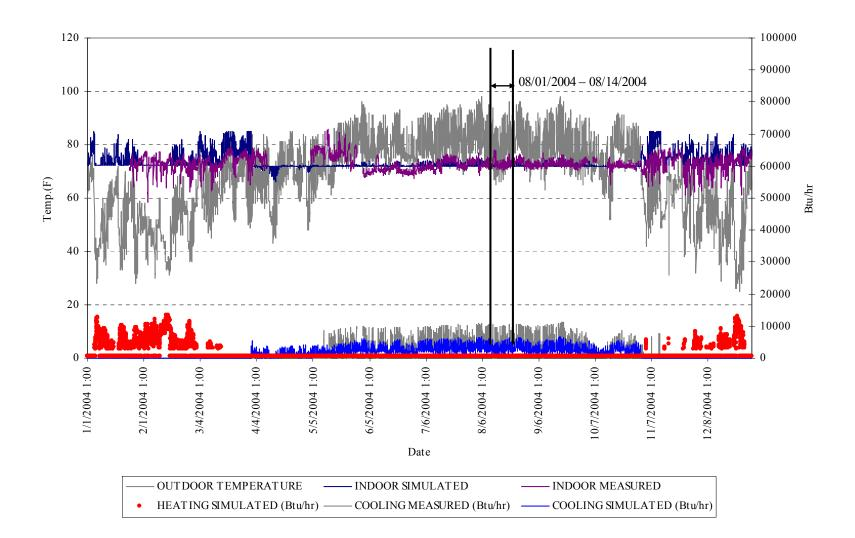
Figure 5.50 Temperature and cooling energy plots without duct model for the whole year
