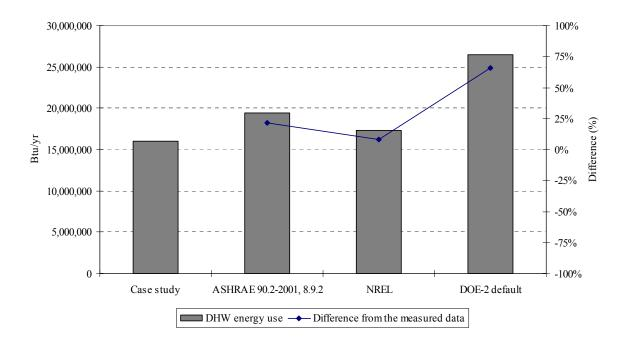
Figure 5.62 Comparison of DHW energy use (pilot light = 600 Btu/hr)
