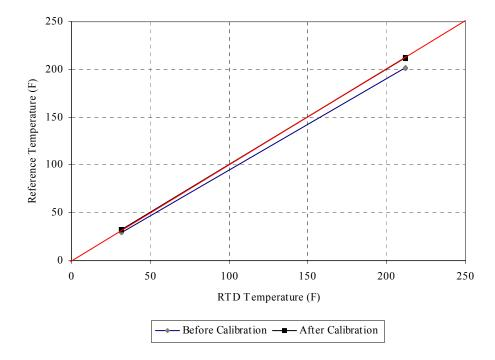
Figure A.3 Calibration of the RTD sensor (Before and after calibration)
