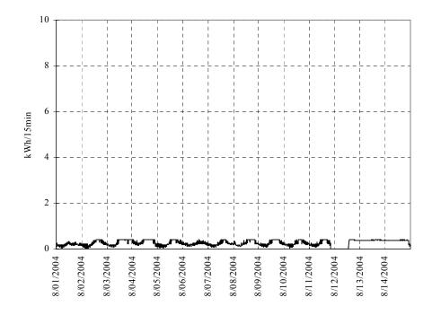
Figure 4.22 Electricity use for the air conditioner blower (CH4153)
