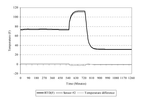
Figure A.12 Time series and residual plot of the RTD sensor and sensor #2 after calibration
