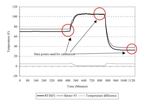
Figure A.15 Time series and residual plot of the RTD sensor and sensor #3 before calibration
