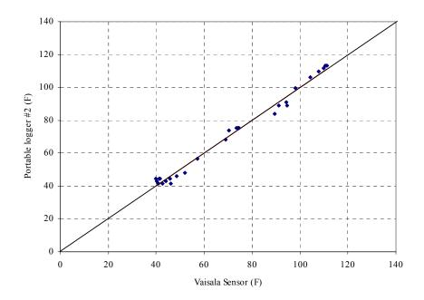
Figure A.54 Comparison of portable data logger #2 and Vaisala sensor after calibration.
