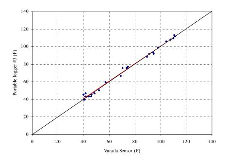
Figure A.56 Comparison of portable data logger #3 and Vaisala sensor before calibration.
