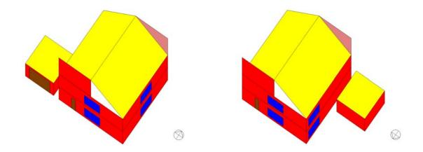
Figure 4.70 DrawBDL views of the code compliant two-story house with detached garage and attic space
