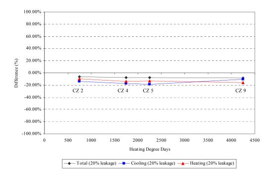
Figure 6.96 Percent difference according to HVAC location (the attic space vs. the conditioned space (20% duct leakage rate))
