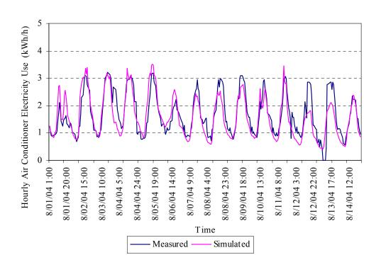
Figure 5.56 Cooling energy with good A/C curve from Henderson et al. (2000)
