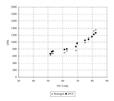
Figure 5.17 Comparison between the IECC and strategy #6 of electricity
