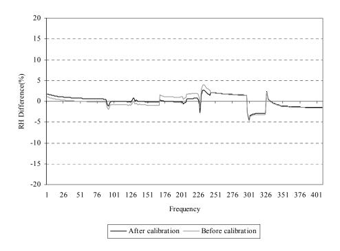
Figure A.33 Residual plot before and after calibration
