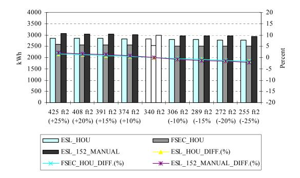
Figure I.1 The variation of supply duct area and results
