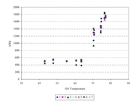
Figure 5.73 Monthly electricity use from the measured data of the case-study house and DOE-2 simulations vs. average monthly outdoor temperature
