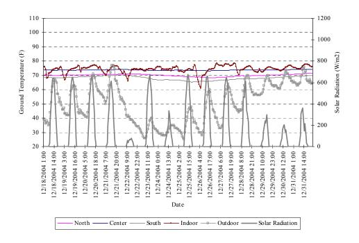
Figure 5.65 Three ground temperatures versus solar radiation for winter period
