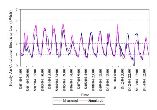
Figure 5.58 Cooling energy with poor A/C curve from Henderson et al. (2000)
