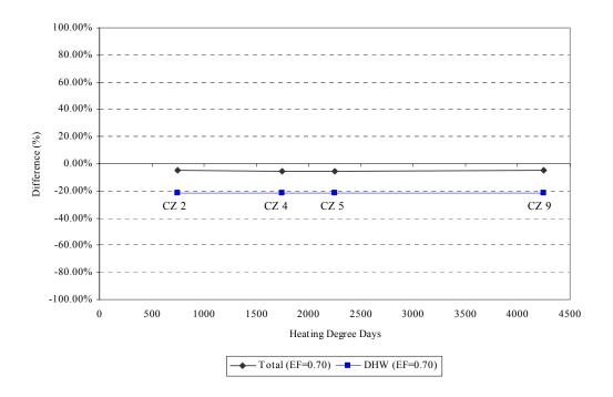
Figure 6.88 Percent difference of annual energy use (base case (0.55 EF) vs. 0.70 EF)
