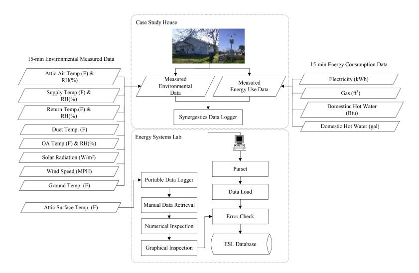
Figure 4.18 Procedure for collecting data
