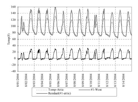
Figure 4.35 West side of inside roof surface temperature
