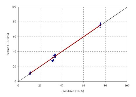
Figure A.32 Comparison of sensor #1 against calculated RH after calibration
