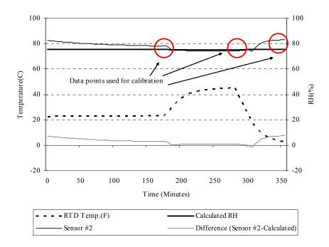
Figure A.36 Time series and residual plot of sensor #2 and calculated RH for Sodium Chloride before calibration
