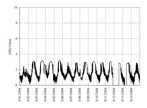
Figure 4.21 Electricity use for the air conditioner (CH4152)
