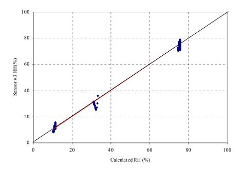
Figure A.44 Comparison of sensor #3 against calculated RH after calibration
