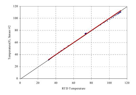
Figure A.13 Comparison of sensor #2 against RTD temperature after calibration
