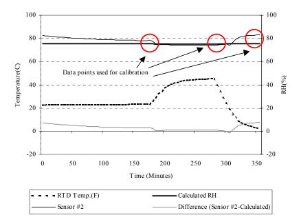
Figure A.40 Time series and residual plot of sensor #3 and calculated RH for Lithium Chloride before calibration
