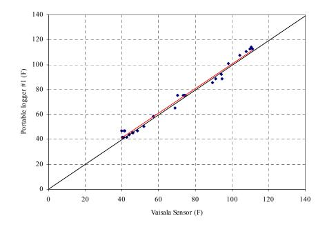
Figure A.51 Comparison of portable data logger #1 and Vaisala sensor after calibration.
