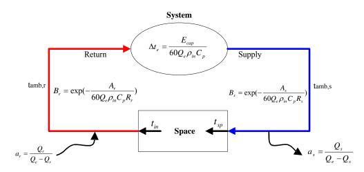
Figure B.1 Schematic diagram of duct model (ASHRAE 152-2004)
