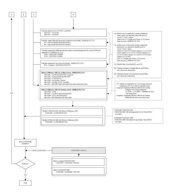
Figure 4.54 Diagram of DOE-2 FUNCTION command for ASHRAE 152-2004 duct loss model (b)
