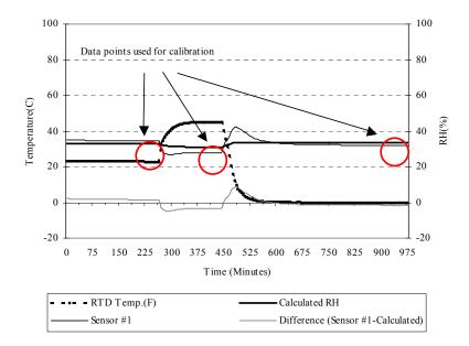
Figure A.29 Time series and residual plot of sensor #1 and calculated RH for Magnesium Chloride before calibration
