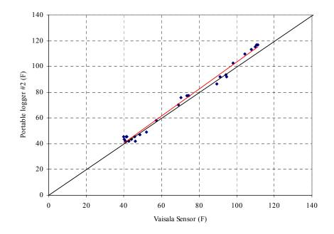
Figure A.53 Comparison of portable data logger #2 and Vaisala sensor before calibration.
