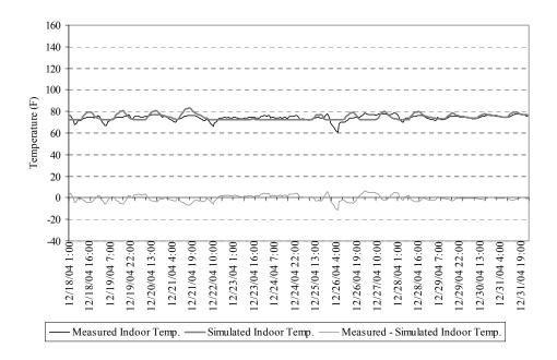
Figure 5.48 The calibrated simulation (run #9) and measured results of the indoor temperature for the period December 18 to December 31, 2004
