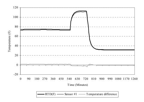
Figure A.7 Time series and residual plot of the RTD sensor and sensor #1 after calibration
