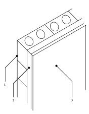
Figure 4.77 8" concrete block wall with perlite fill
