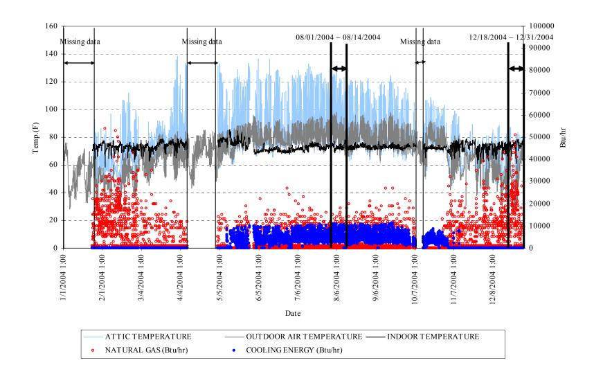
Figure 5.24 Measured attic, indoor, outdoor temperature, and heating and cooling energy
