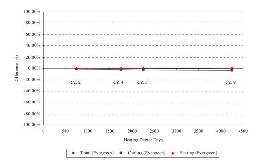
Figure 6.104 Percent difference of annual energy use (base case (no shading) vs. west side shading of evergreen))
