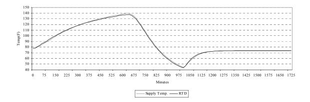
Figure A.67 Time series plot of supply sensor vs. RTD sensor
