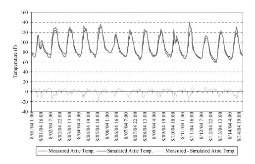
Figure 5.42 The calibrated simulation (run #9) and measured results of the attic temperature for the period August 1 to August 14, 2004
