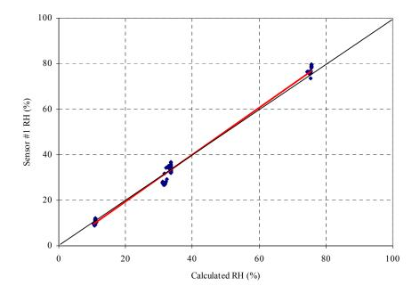
Figure A.31 Comparison of sensor #1 against calculated RH before calibration
