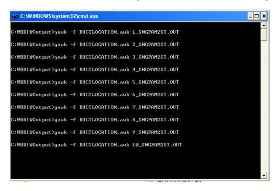
C.5. Batch file run to extract data using commands of GAWK from DOE-2 output
