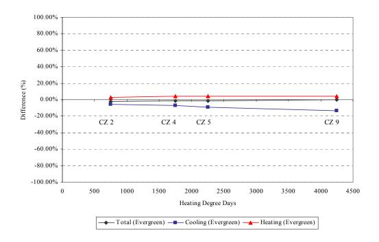
Figure 6.108 Percent difference of annual energy use (base case (no shading) vs. both (east and west) side shading of evergreen))
