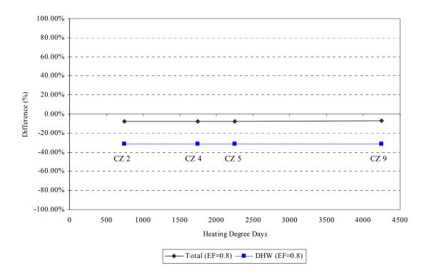
Figure 6.90 Percent difference of annual energy use (base case (0.55 EF) vs. 0.80 EF)
