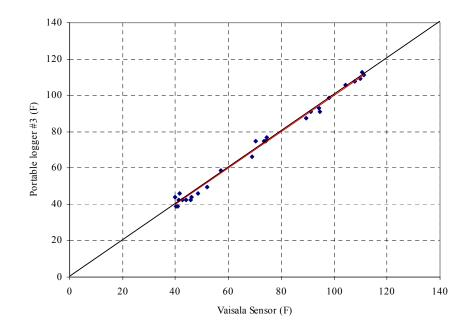
Figure A.57 Comparison of portable data logger #3 and Vaisala sensor after calibration.
