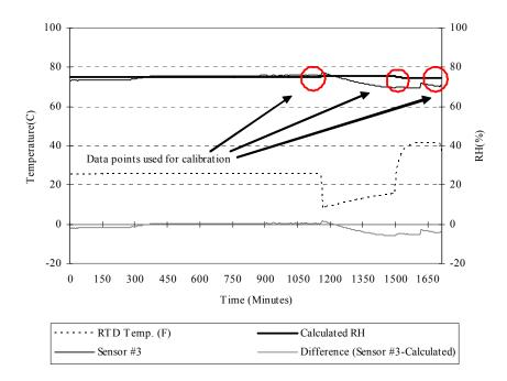
Figure A.42 Time series and residual plot of sensor #3 and calculated RH for Sodium Chloride before calibration
