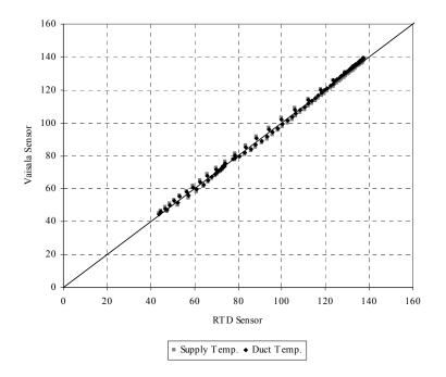
Figure A.65 RTD sensor temperature vs. Vaisala temperature sensor
