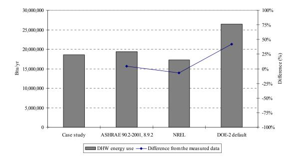
Figure 5.61 Comparison of DHW energy use (pilot light = 300 Btu/hr)
