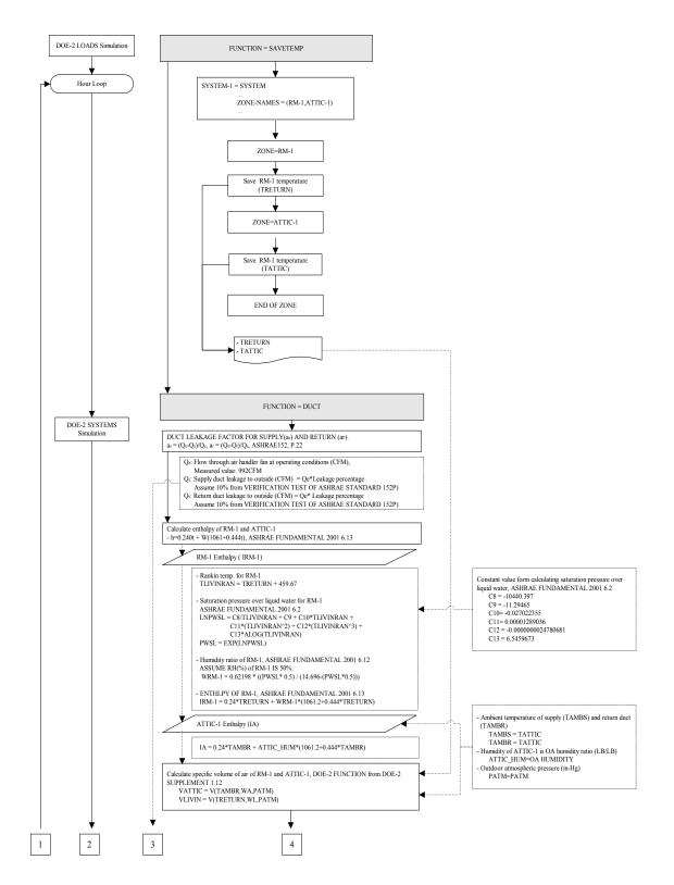
Figure B.2 Diagram of DOE-2 FUNCTION command for ASHRAE 152-2004 duct loss model (a)
