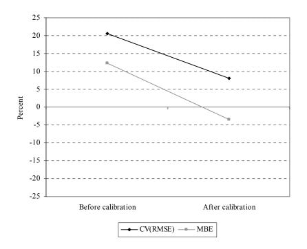
Figure A.64 CV(RMSE) and MBE plot before and after calibration.
