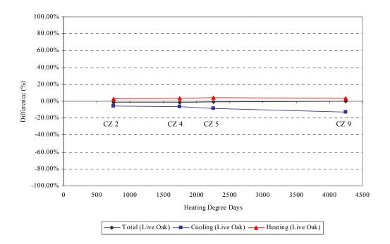
Figure 6.106 Percent difference of annual energy use (base case (no shading) vs. both (east and west) side shading of live oak))
