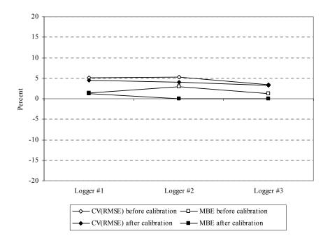
Figure A.59 CV(RMSE) and MBE plot before and after calibration.
