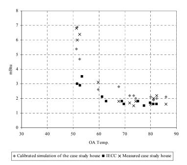
Figure 5.6 Measurement and calibration results of the natural gas
