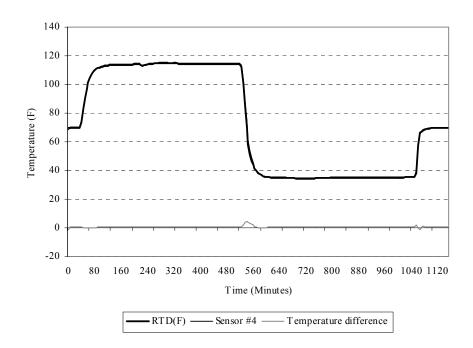
Figure A.22 Time series and residual plot of the RTD sensor and sensor #4 after calibration
