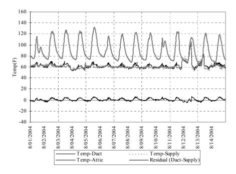
Figure 4.33 Supply, attic and duct temperature (CH3802, CH3812, CH3806)
