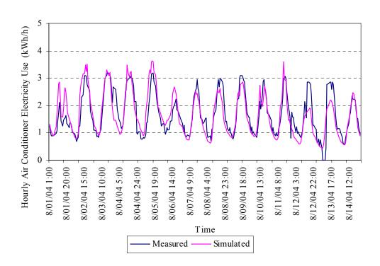
Figure 5.57 Cooling energy with typical A/C curve from Henderson et al. (2000)
