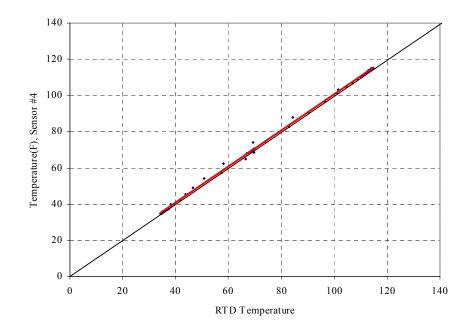
Figure A.23 Comparison of sensor #4 against RTD temperature after calibration
