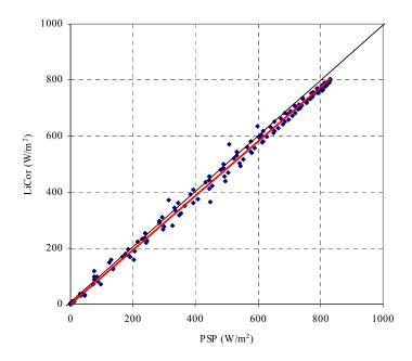
Figure A.63 PSP versus Li-Cor after calibration.
