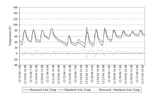
Figure 5.47 The calibrated simulation (run #9) and measured results of the attic temperature for the period December 18 to December 31, 2004
