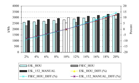
Figure I.5 The variation of supply duct leakage and results
