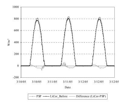
Figure A.62 PSP and Li-Cor time series plot after calibration.
