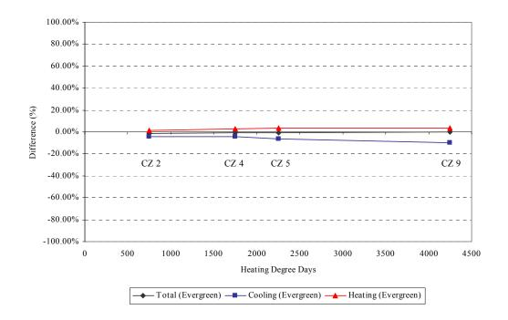
Figure 6.100 Percent difference of annual energy use (base case (no shading) vs. east side shading of evergreen))
