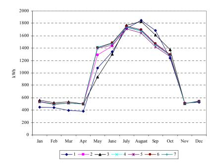
Figure 5.72 Monthly electricity use from the measured data of the case-study house and DOE-2 simulations
