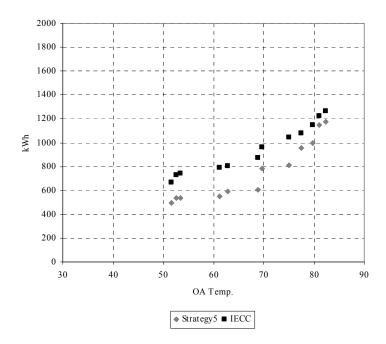
Figure 5.15 Comparison between the IECC and strategy #5 of electricity
