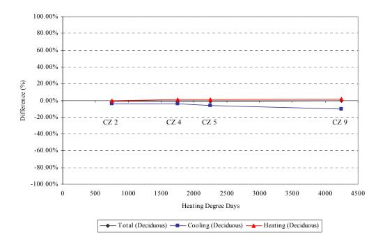
Figure 6.99 Percent difference of annual energy use (base case (no shading) vs. east side shading of deciduous tree))
