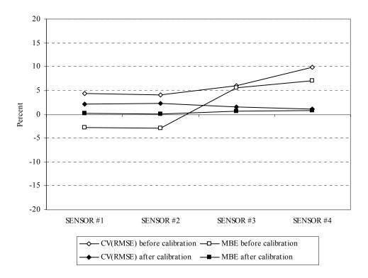
Figure A.27 CV(RMSE) and MBE plot before and after calibration.
