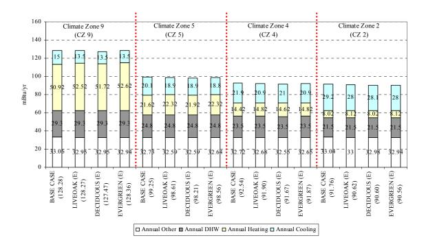
Figure 6.101 Annual energy use of east side tree shading
