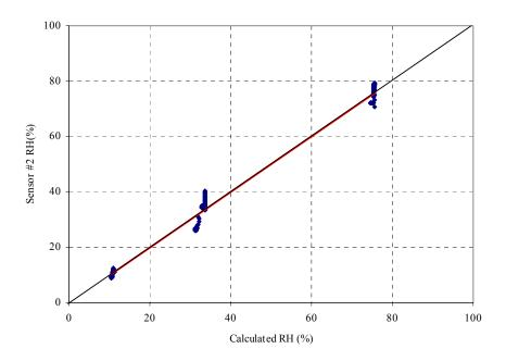
Figure A.38 Comparison of sensor #2 against calculated RH after calibration
