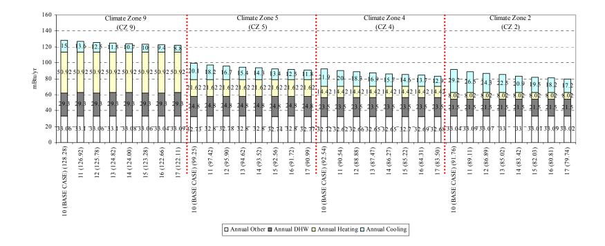
Figure 6.77 Annual energy use of different air conditioner efficiency
