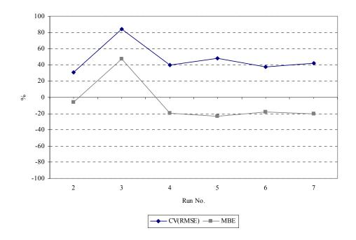
Figure 5.75 CV (RMSE) and MBE of natural gas uses
