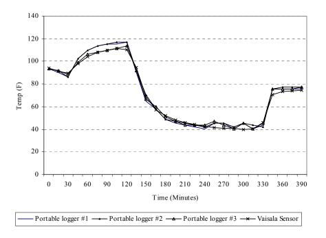
Figure A.49 Temperature plots of the three Onset portable data loggers versus the Vaisala sensor
