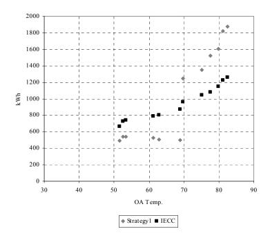
Figure 5.7 Comparison between the IECC and strategy #1 of electricity
