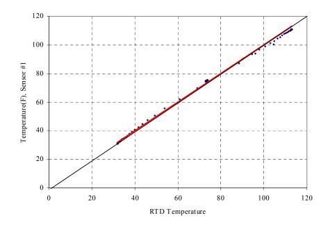
Figure A.8 Comparison of sensor #1 against RTD temperature after calibration
