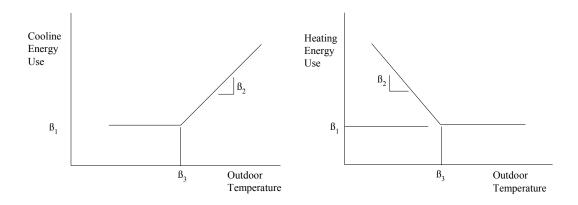
Figure 4.45 IMT three parameter change-point models
