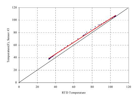
Figure A.16 Comparison of sensor #3 against RTD temperature before calibration
