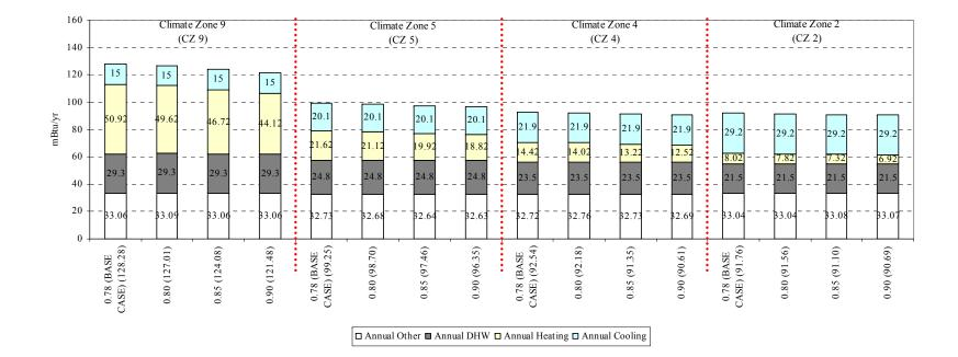
Figure 6.81 Annual energy use of different gas furnace efficiency
