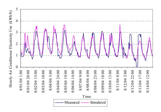
Figure 5.55 Cooling energy with old DOE-2.1e A/C curve (old SDL-C17)
