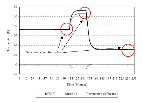
Figure A.5 Time series and residual plot of the RTD sensor and sensor #1 before calibration
