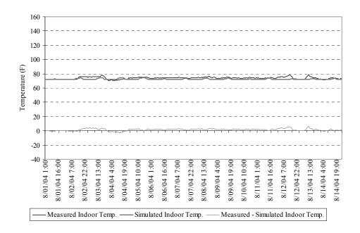
Figure 5.43 The calibrated simulation (run #9) and measured results of the indoor temperature for the period August 1 to August 14, 2004
