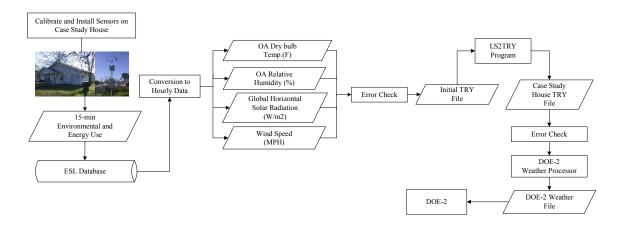
Figure 4.46 Flowchart of the DOE-2 weather data processing
