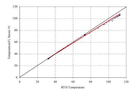
Figure A.6 Comparison of sensor #1 against the RTD sensor before calibration
