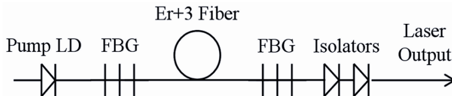
Figure 28. Experimental setup for fiber laser used as the light source in Yuma, AZ field tests
