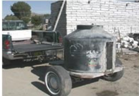
Fig. 3. Tow mixer (Fuller 2004)
