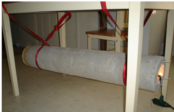
Fig. 15. Thermal conductivity test
