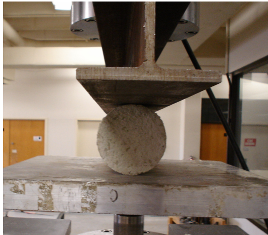
Fig. 10. Split cylinder tensile test
