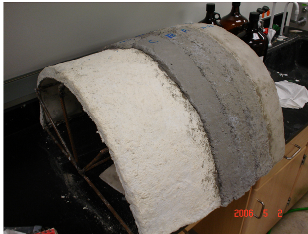
Fig. 39. Concrete layer on papercrete
