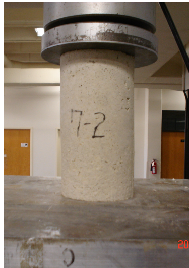
Fig. 6. Cylinder compression test
