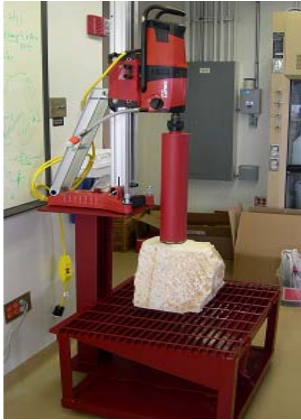
Figure 3.11: Heavy duty HILTI DD200 Core Press and Core Bit (J. Nevito 15 )
