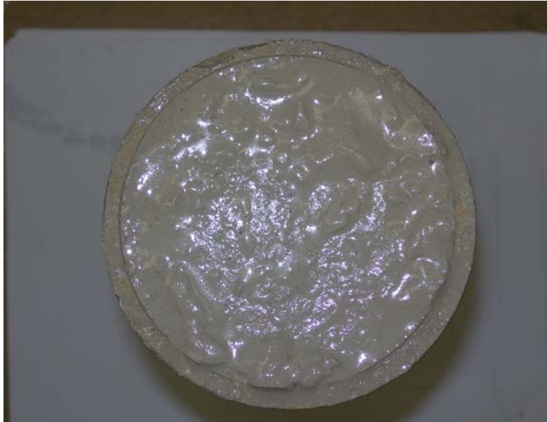
Figure D.1: Core with just formed filter-cake-1
