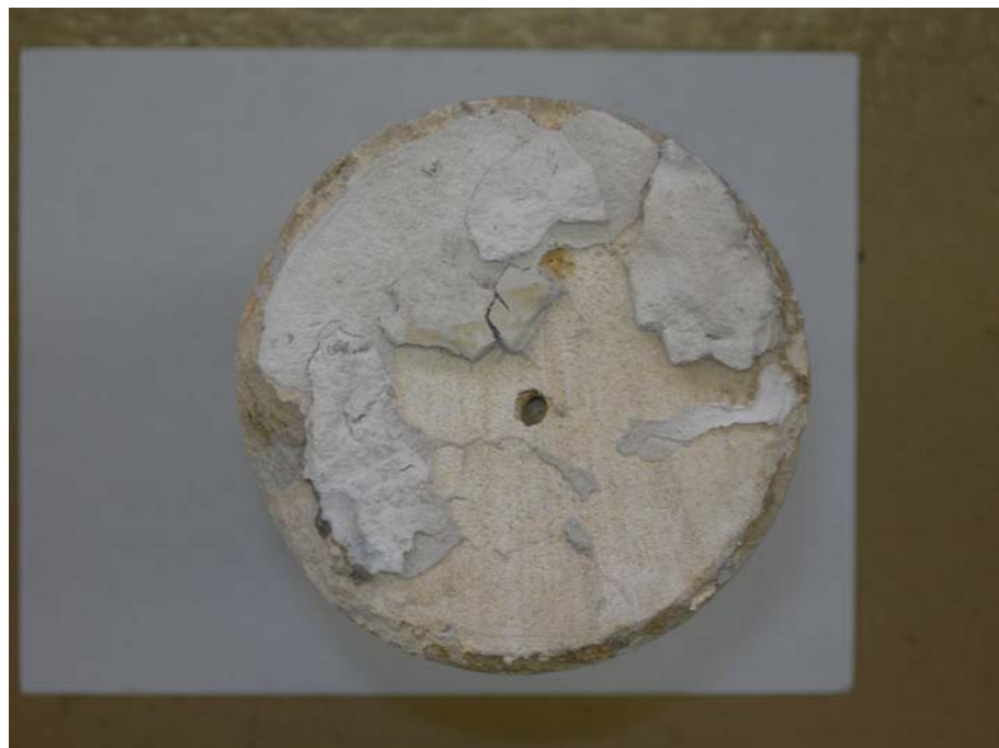
Figure 4.23: Core with mud cake after acid jetting ( q=100 cc/min, duration 45 sec, reverse circulation after jetting)
