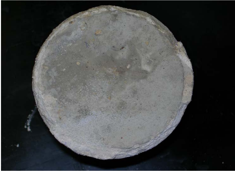
Figure 4.12: Core with mud cake after water jetting ( q=100 cc/min, duration 90 sec)
