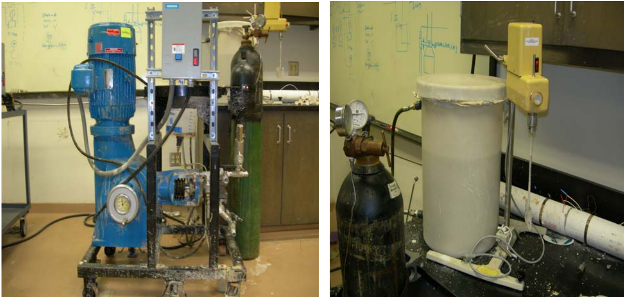
Figure 3.10: Mud pump with backpressure nitrogen vessel; mud tank with mud mixer
