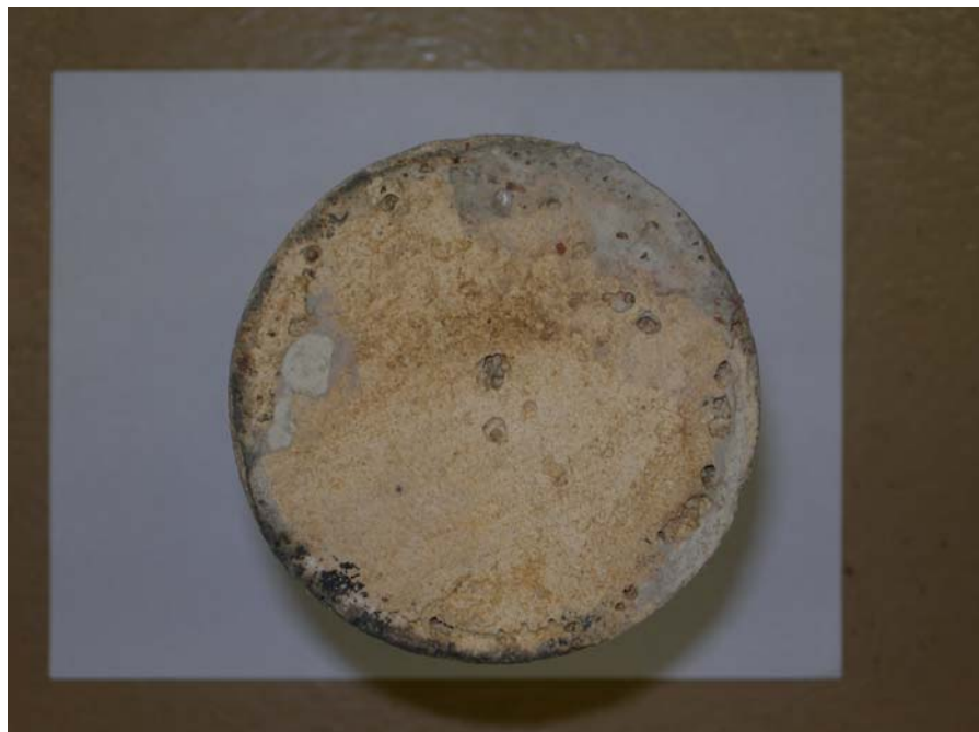
Figure 4.21: Core with mud cake after acid jetting ( q=100 cc/min, duration 90 sec, reverse circulation after jetting)
