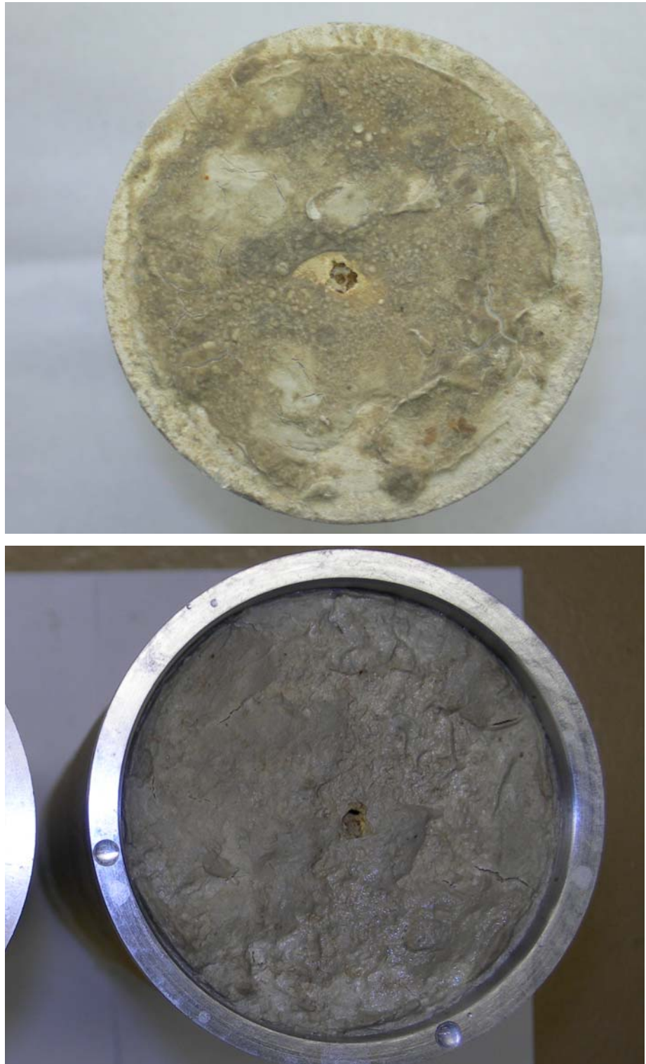
Figure 4.5: The upper core was subject to acid jetting ( q=100 cc/min, duration 60 second), the lower one was subject to acid for 20 second ( q is 100 cc/min)
