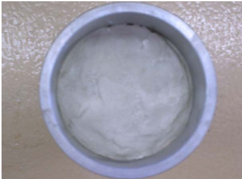
Figure D.2: Core with just formed filter-cake-2
