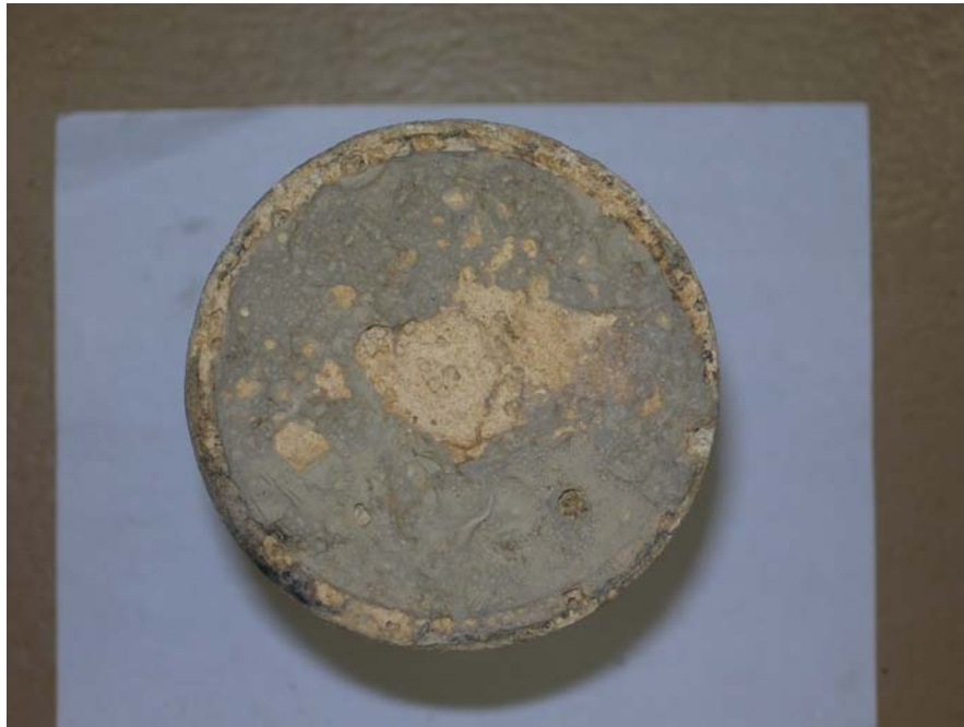
Figure 4.20: Core with mud cake after acid jetting ( q=140 cc/min, duration 60 sec)
