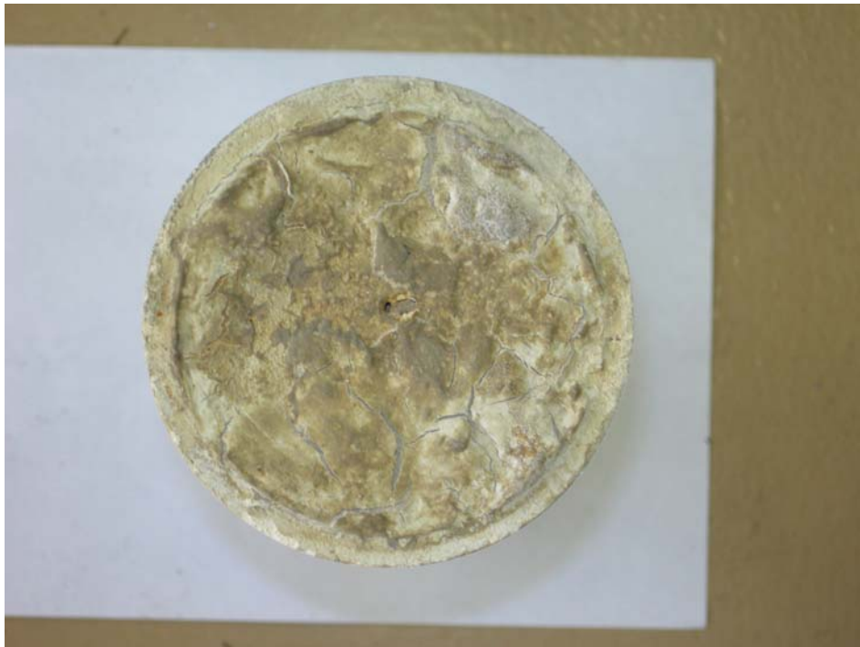
Figure 4.13: Core with mud cake after acid jetting ( q=100 cc/min, duration 20 sec)
