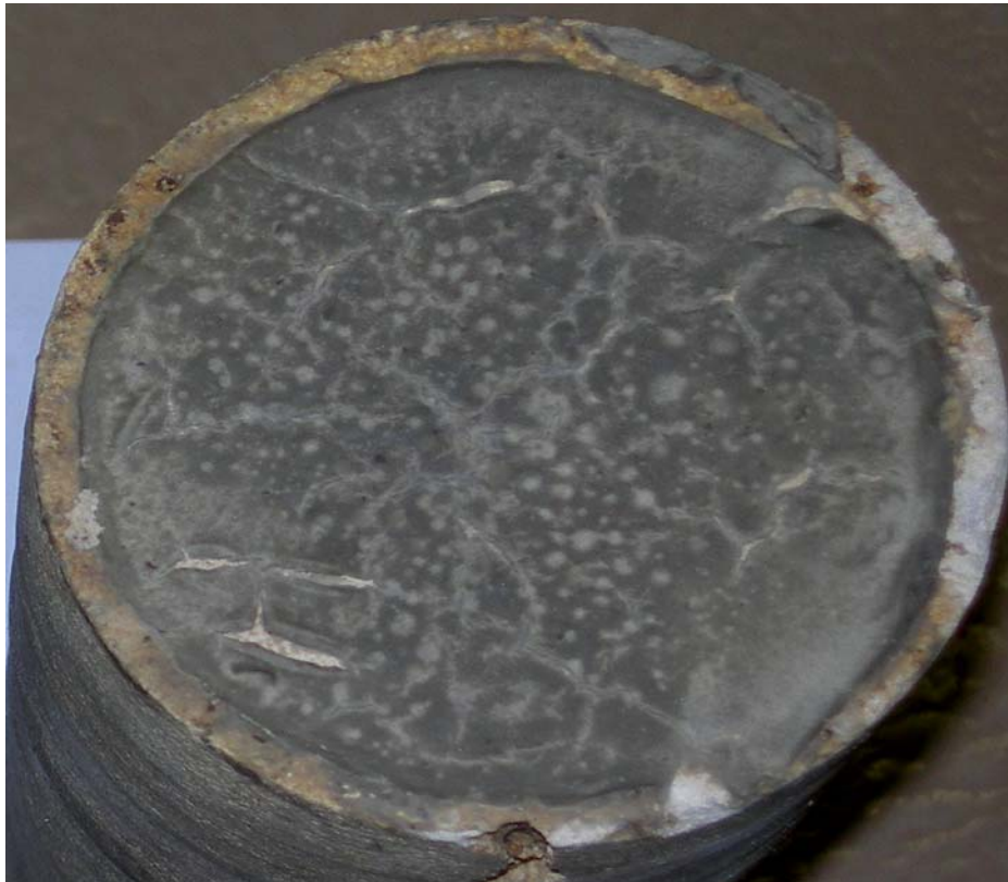
Figure 4.18: Dry filter-cake (exposed to the open air for 24 hrs after deposition)
