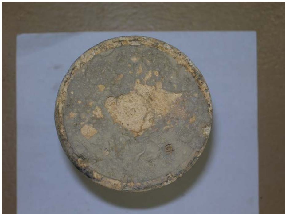
Figure 4.9: Core with mud cake after acid jetting ( q=140 cc/min, duration 60 sec)
