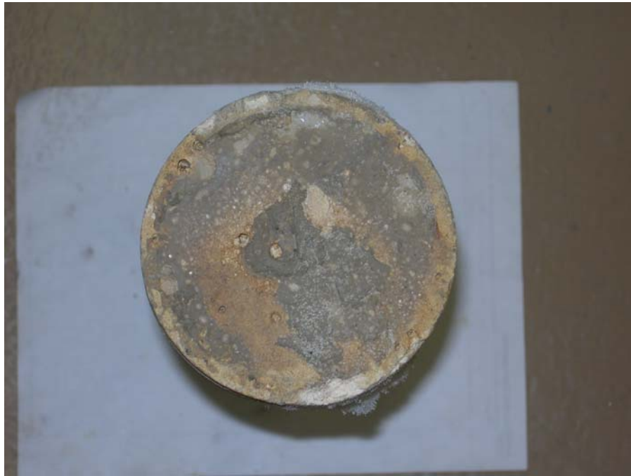
Figure 4.22: Core with mud cake after acid jetting ( q=140 cc/min, duration 90 sec)
