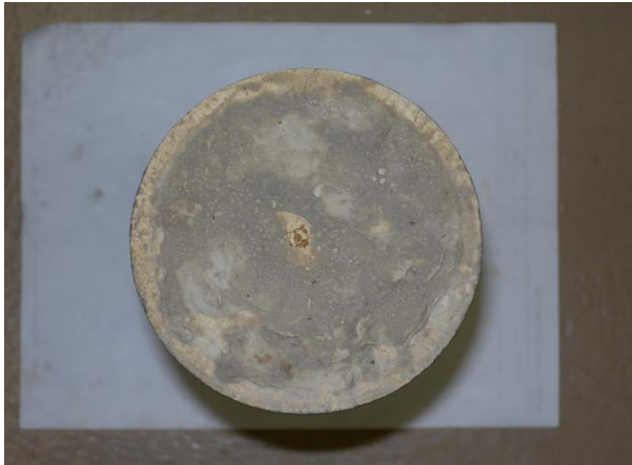
Figure 4.8: Core with mud cake after acid jetting ( q=100 cc/min, duration 60 sec)
