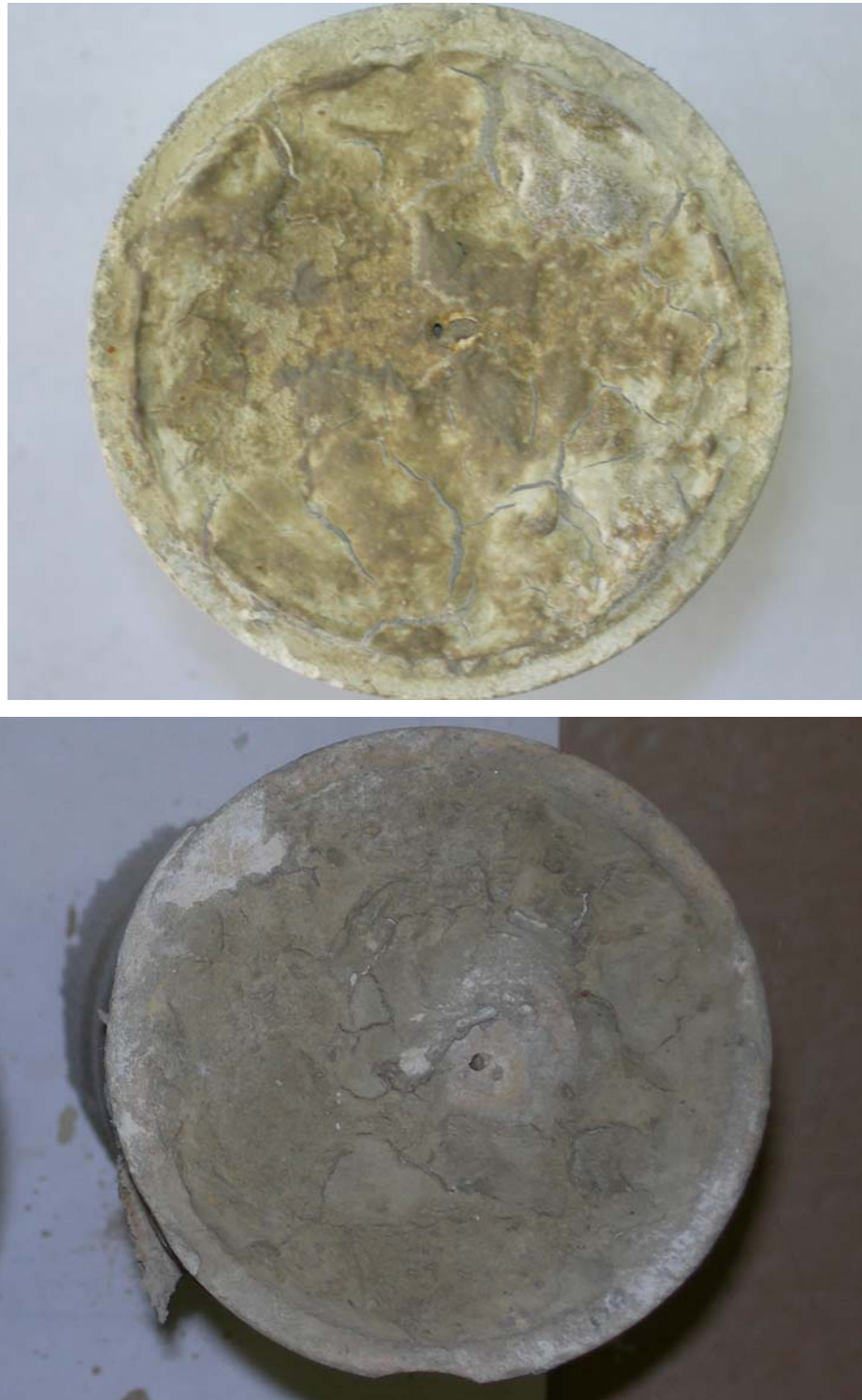
Figure 4.19: Two acid jetted cores; one jetted immediately, the other after 24 hours of drying out.
