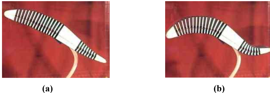
(a) (b) Fig. 7. Adaptive wings: (a) straight wing, (b) bent wing (adapted from Smart Material Products, 2006)
