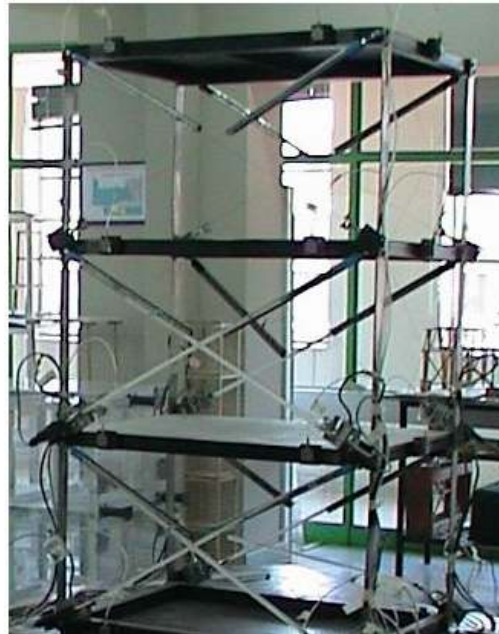
Fig. 25. Three story structure with SMA wires and sensors
