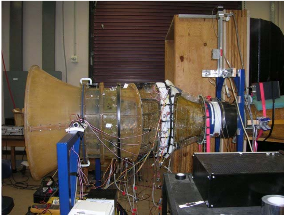
Figure 13: Experimental Setup for Duct Testing
