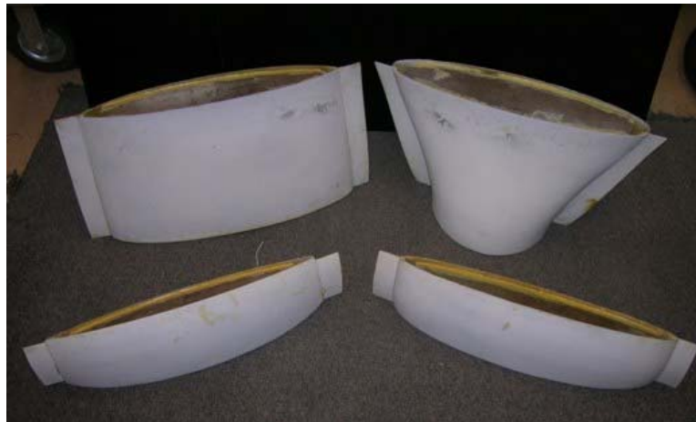
Figure 4: Molds Employed to Create Fiberglass Reproductions of the Inlet Duct
