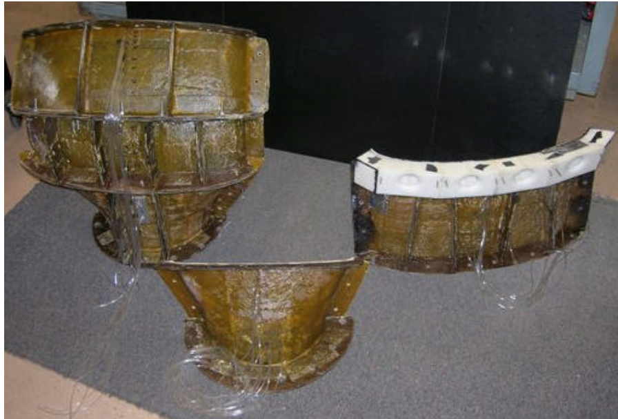
Figure 15: Fiberglass duct section with flow actuators
