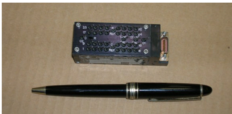
Figure 17: Electronically scanning pressure sensors
